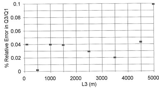
**Figure 9** Percentage relative error in simulating  $Q_3/Q_1$  for the second investigated case
