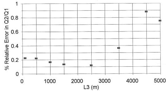
**Figure 5** Percentage relative error in simulating  $Q_2/Q_1$  for the first investigated case
