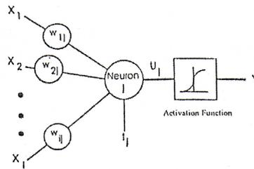
**Figure 2** Typical picture of a model neuron that exists in every neural network
