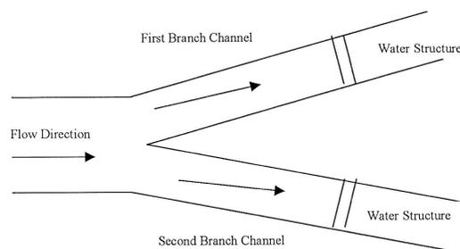
**Figure 1** Schematic diagram for the investigated channels junction
