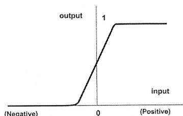
**Figure 3** The Sigmoid activation function used in designed networks
