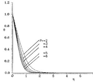
**Figure 16** The variation of the dimensionless temperature  $\theta$  with  $Pr$  for  $N = 3$ ,  $Sc = 10$ ,  $\alpha = -0.4$ ,  $\beta_1 = 0.12$ ,  $\beta_2 = 0.1$ ,  $Pr = 2, 3, 4, 5, 6$
