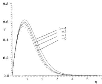
**Figure 5** The variation of the dimensionless velocity  $\phi'$  with  $\beta_1$  for  $Pr = 0.73$ ,  $Sc = 1.4$ ,  $N = 3$ ,  $\beta_2 = 3.0$ ,  $\alpha = -0.4$ ,  $\beta_1 = 0, 1, 2, 4$
