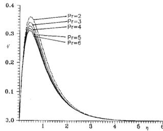
**Figure 15** The variation of the dimensionless velocity  $\phi'$  with  $Pr$  for  $N = 3$ ,  $Sc = 10$ ,  $\beta_1 = 0.12$ ,  $\alpha = 0.6$ ,  $\beta_2 = 0.1$ ,  $Pr = 2, 3, 4, 5, 6$
