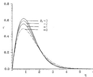
**Figure 8** The variation of the dimensionless velocity  $\phi'$  with  $\beta_2$  for  $Pr = 0.73$ ,  $Sc = 1.4$ ,  $N = 3$ ,  $\beta_1 = 4.0$ ,  $\alpha = -0.4$ ,  $\beta_2 = 0, 1, 2, 3$
