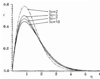
**Figure 17** The variation of the dimensionless velocity  $\phi'$  with  $Sc$  for  $N = 3$ ,  $Pr = 4$ ,  $\beta_1 = 0.12$ ,  $\alpha = 0.6$ ,  $\beta_2 = 0.1$ ,  $Sc = 2, 5, 7, 10$
