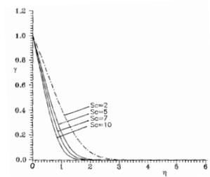
**Figure 18** The variation of the dimensionless concentration  $\gamma$  with  $Sc$  for  $N = 3$ ,  $Pr = 4$ ,  $\beta_1 = 0.12$ ,  $\beta_2 = 0.1$ ,  $\alpha = 0.6$ ,  $Sc = 2, 5, 7, 10$
