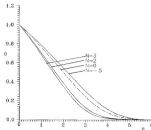
**Figure 12** The variation of the dimensionless temperature  $\theta$  with  $N$  for  $Pr = 0.73$ ,  $Sc = 1.4$ ,  $\alpha = -0.4$ ,  $\beta_2 = 3.0$ ,  $N = -0.5, 0, 1, 2, 3$
