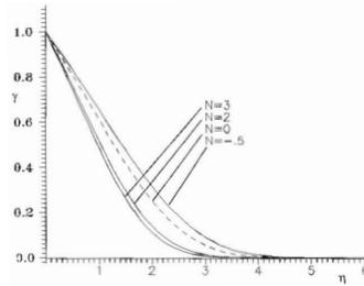
**Figure 13** The variation of the dimensionless concentration  $\gamma$  with  $N$  for  $Pr = 0.73$ ,  $Sc = 1.4$ ,  $\beta_2 = 3.0$ ,  $N = -0.5, 0, 1, 2, 3$
