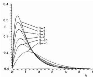
**Figure 14** The variation of the dimensionless velocity  $\phi'$  with  $N$  for  $Pr = 4$ ,  $Sc = 10$ ,  $\beta_2 = 0.1$ ,  $\alpha = 0.6$ ,  $\beta_2 = 0.1$ ,  $N = -1, -0.5, 0, 1, 2, 3$
