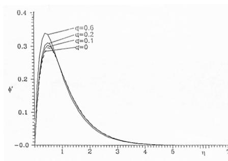
**Figure 2** The variation of the dimensionless velocity  $\phi'$  with  $\alpha$  for  $Pr = 0.73$ ,  $Sc = 1.4$ ,  $N = 3$ ,  $\beta_1 = 4.0$ ,  $\beta_2 = 3.0$ ,  $\alpha = -0.1, -0.2, -0.3, 0.4$
