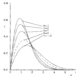
**Figure 11** The variation of the dimensionless velocity  $\phi'$  with  $N$  for  $Pr = 0.73$ ,  $Sc = 1.4$ ,  $\beta_1 = 4.0$ ,  $\alpha = -0.4$ ,  $\beta_2 = 3.0$ ,  $N = -0.5, 0, 1, 2, 3$
