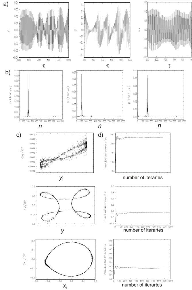
**Figure 6** Time history (a) , power spectral density (FFT) (b), Poincaré map (c) and maximum Lyapunov exponent(d) corresponding to coordinates  $y_1$  , $x_1$  and  $\varphi$  for:  $\beta_1 = 0.5$ ,  $\beta_2 = 2$ ,  $d = 0.02$ ,  $\gamma_1 = 0$ ,  $\gamma_2 = 0.0002$ ,  $q = 0.0005$ ,  $\mu = 1.07$
