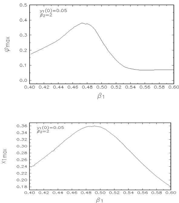
**Figure 3** Amplitudes of the pendulum versus frequency ratio  $\beta_1$  (internal resonant curves) for  $y_1(0) = 0.05$  and  $d = 0.02$ ,  $\beta_2 = 2$ ,  $\gamma_1 = \gamma_2 = 0$ ,  $q = 0$
