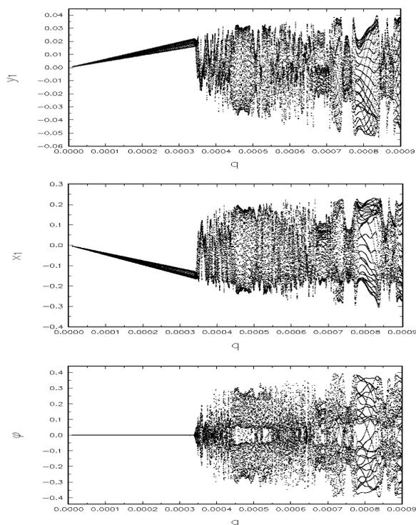
**Figure 5** Bifurcation diagram for  $y_1$ ,  $x$  and  $\varphi$  for  $\beta_1 = 0.5$ ,  $\beta_2 = 2$ ,  $d = 0.02$ ,  $\gamma_2 = 0.002$ ,  $\mu_1 = 1.07$
