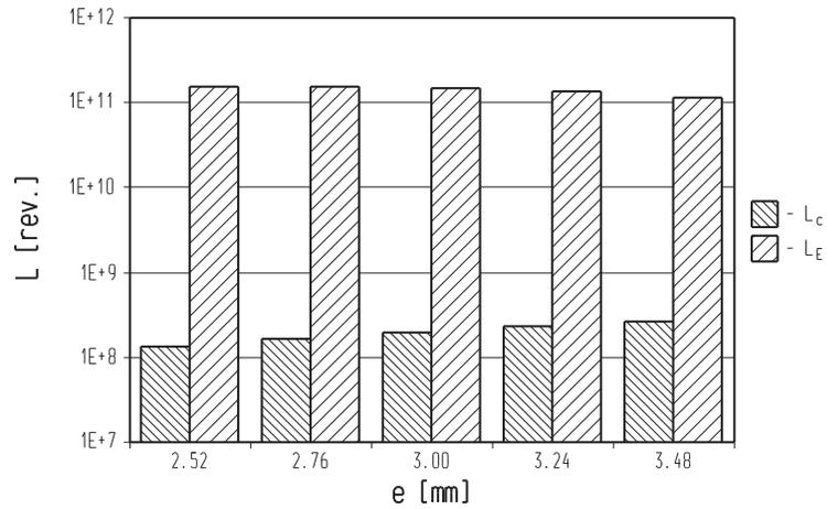
**Figure 9** Fatigue life of the central roller bearing  $L_c$  and the meshing of the Cyclo gear  $L_E$  for different values of  $e$  and the most advantageous values of  $D_e = D_{e\ opt}$
