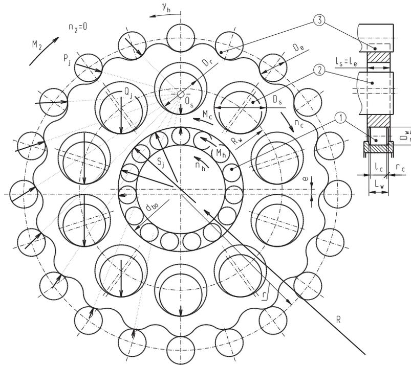
**Figure 1** Operation principle and state of load in power transmission system of the cycloidal gear
