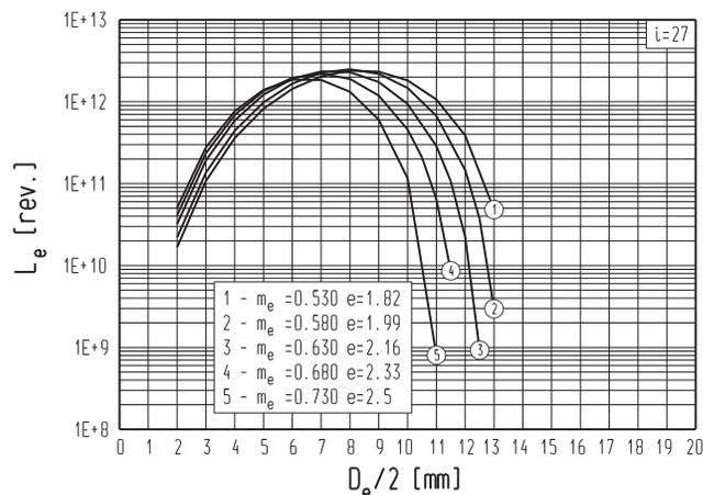
**Figure 5** Fatigue life of single tooth  $L_e$  of the planetary wheel in function of radius of the roller of co-operating wheel,  $i = 27$
