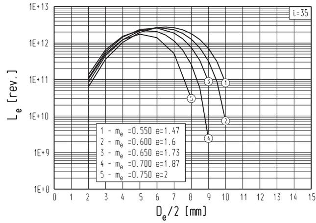
**Figure 6** Fatigue life of single tooth  $L_e$  of the planetary wheel in function of radius of the roller of co-operating wheel,  $i = 35$
