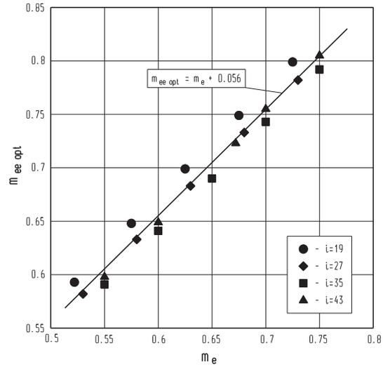
**Figure 8** Optimal value of the curtailment coefficient of epicycloid equidistant  $m_{ee\ opt}$  versus curtailment coefficient of epicycloid  $m_e$
