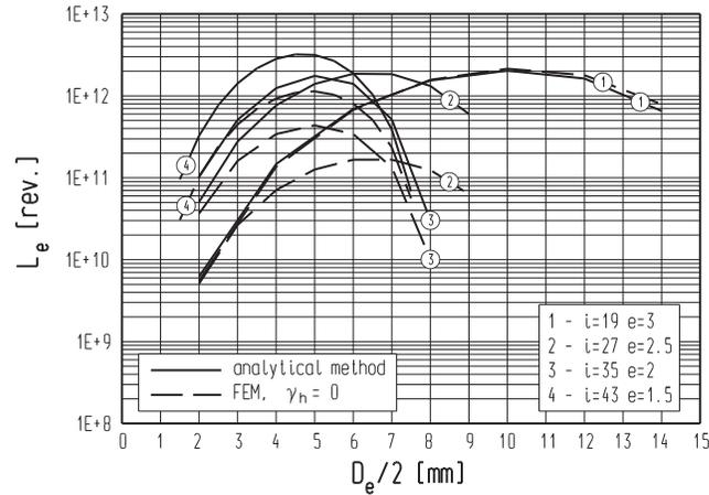
**Figure 3** Comparison of fatigue life calculation results of single tooth for load distribution obtained according to analytical and FEM methods
