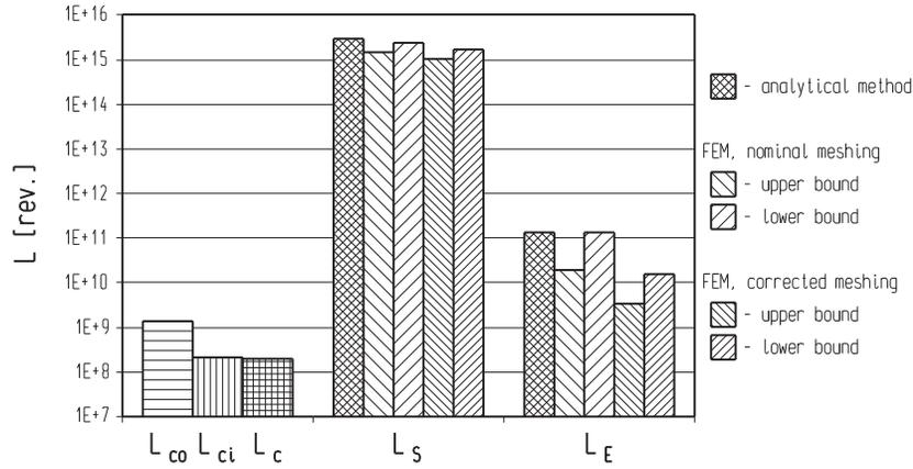
Figure 2 Durability of rolling pairs of Cyclo gear
