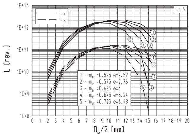
**Figure 4** Fatigue life of single tooth  $L_e$  of the planetary wheel and the meshing of Cyclo gear  $L_E$  in function of radius of the roller of co-operating wheel,  $i = 19$
