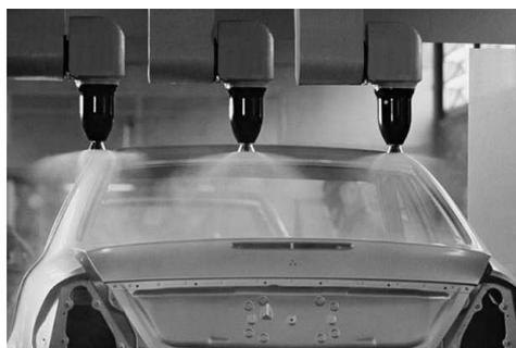
**Figure 14** The process of nanolaquer application in the factory of *Mercedes-Benz*
