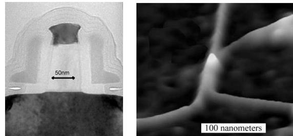
**Figure 15** Transistors made in new Intel proces
