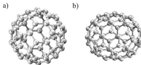
**Figure 4** Structure of fullerene: a) C60, b) C70
