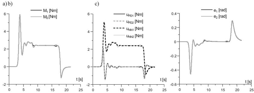
**Figure 5** Driving torques (a), compensating and PD control (b) and tracking errors (c) for neural control system
