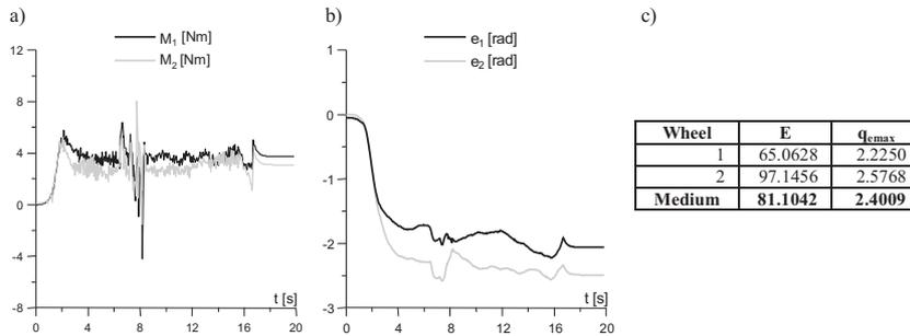
**Figure 11** Driving torques (a), tracking errors (b) and obtained quantitative assess (c) for Pioneer 2DX robot with PD controller
