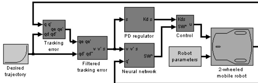
**Figure 4** The diagram of the neural control system for 2-wheeled mobile robot
