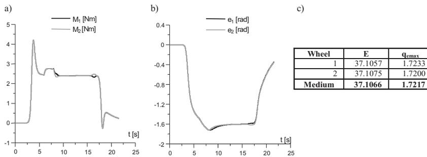
**Figure 7** Driving torques (a), tracking errors (b) and obtained quantitative assess (c) for PD controller
