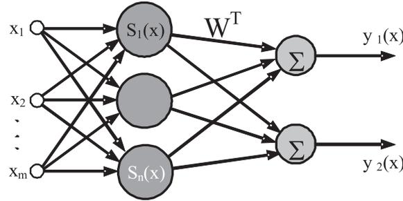
**Figure 2** Neural networks with radial basis functions
