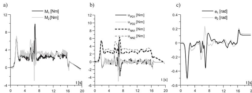
**Figure 9** Driving torques (a), compensating and PD control (b) and tracking errors (c) for Pioneer 2DX robot with neural control system
