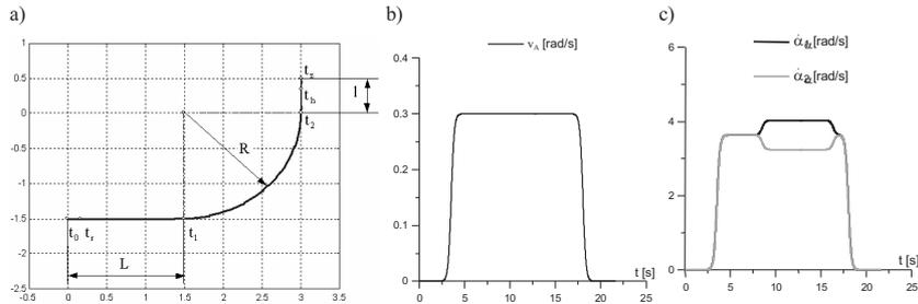
**Figure 3** Desired: motion path of point H (a), speed of point A (b) and velocities of wheels 1 and 2 (c) of mobile robot
