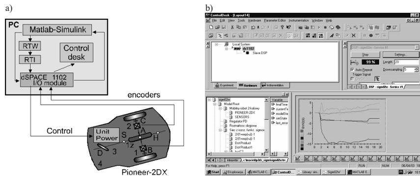
**Figure 8** Experimental environment diagram for Pioneer 2DX rapid prototyping (a) and ControlDesk 1.0 software for experiment managing (b)
