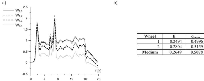
**Figure 10** Selected estimations of robot parameters (a) and obtained quality rates (b) for Pioneer 2DX robot with neural control system
