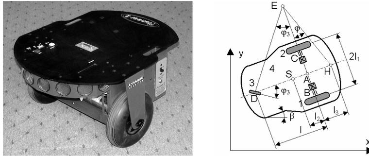
Figure 1 Wheeled mobile robot Pioneer 2DX and its model
