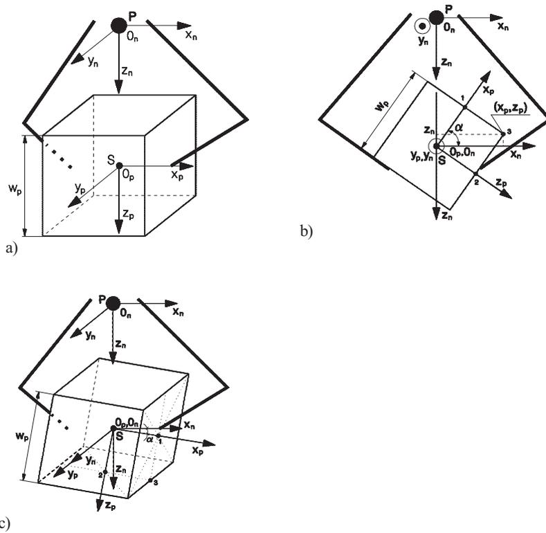
**Figure 4** The manipulator gripping device - manipulated object system. Exemplary selection of local systems of reference for the case of the object manipulated in the form of a homogeneous cube: a) matrix of transformation of local systems of reference according to Eq. (19); b), c) matrix of transformation of local systems of reference according to Eq. (30). The local system of reference of the manipulated object  $(x_p y_p z_p O_p)$  is its main central system of inertia
