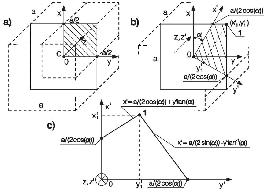
Figure 9 Scheme of transformations of geometrical dimensions in local systems of reference
