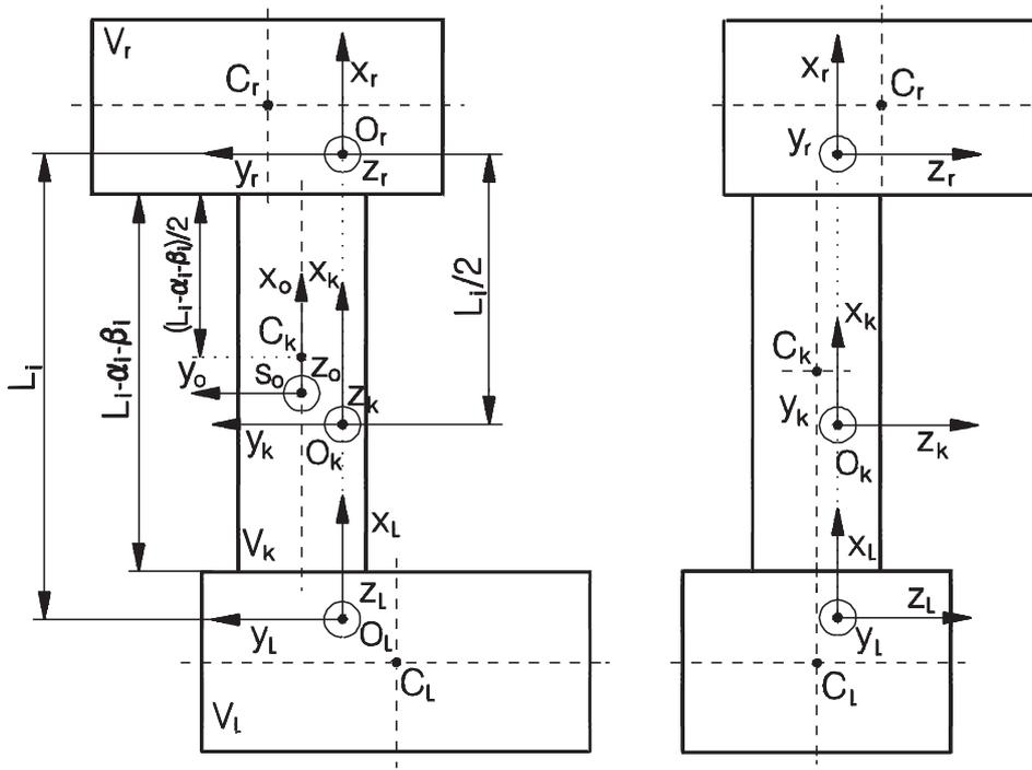
**Figure 7** Design scheme of the  $i$ -th link of the manipulator under analysis. Systems of co-ordinates correspond to links 1 and 2
