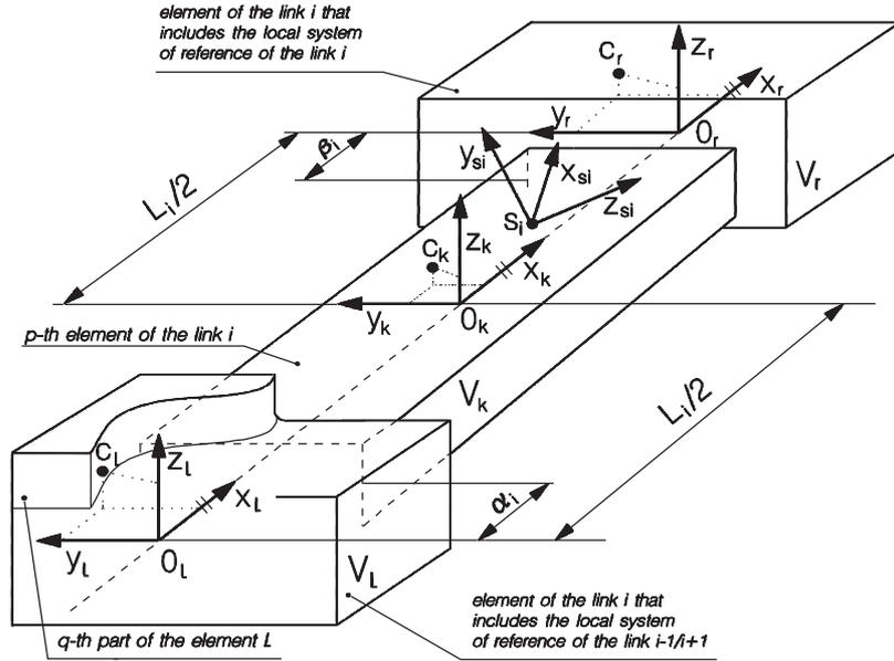
Figure 1 Structural division of the  $i$ -th link of the manipulator
