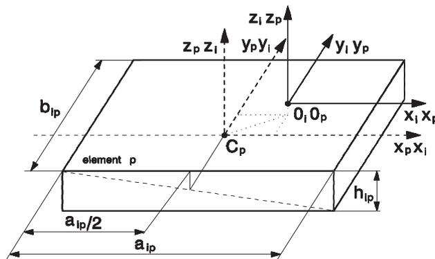
**Figure 6** Shape of the  $p$ -th element of the  $i$ -th link of the exemplary manipulator
