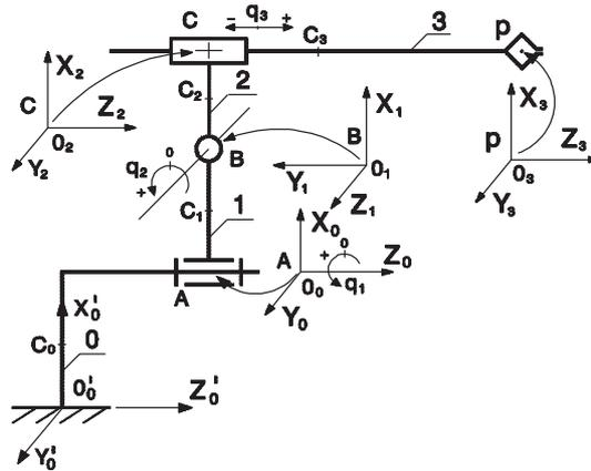
**Figure 5** Kinematic scheme of the *NM7MAR* manipulator. Selection of systems of co-ordinates of links
