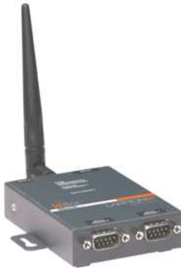
Figure 3 Wireless WiBox serial server
