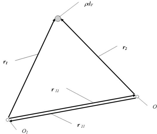
**Figure 5** Position of the elementary mass in space
