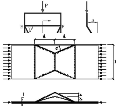
Figure 3 Pitched-roof mechanism
