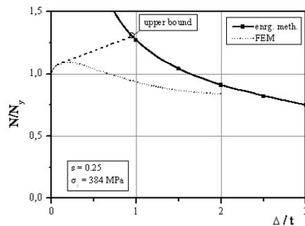
**Figure 9** Loading path of rectangular steel plate of dimension  $1600 \times 800 \times 50$  [mm], (pitched roof mechanism for energy method –  $s = 0.25$ )
