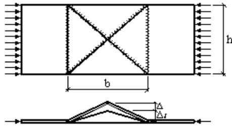
Figure 4 Mechanism type "pyramid" [18]
