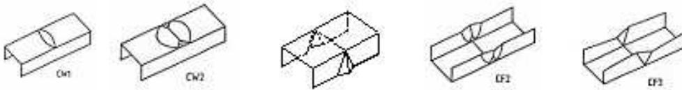
Figure 5 Plastic mechanisms of failure in channel-section column
