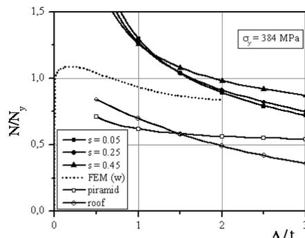
**Figure 7** Loading path and failure curves of rectangular steel plate of dimension  $1600 \times 800 \times 50$  [mm];  $\Delta_i = 0$
