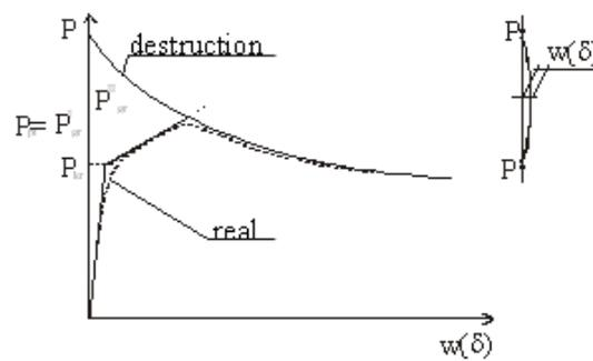
**Figure 2** Thin-walled column subject to eccentric compression. Lower and upper bound estimation of the load-capacity
