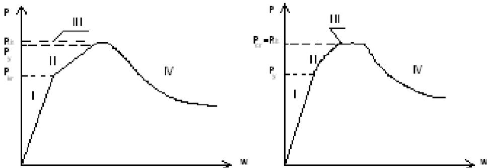
**Figure 1** Load paths of thin-walled beam-column, a) – elastic buckling of the weakest plate element, b) – elasto-plastic buckling of the weakest plate element
