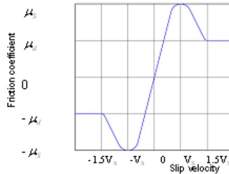
Figure 8 Change of friction coefficient with slip velocity
