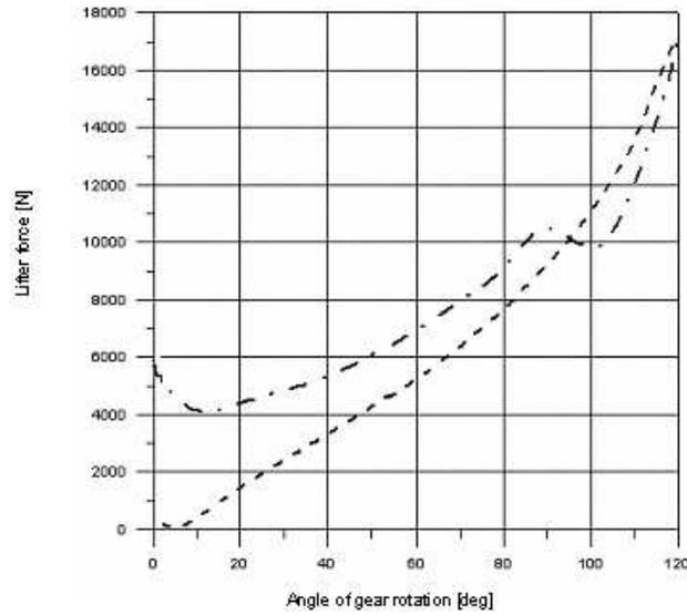
**Figure 4** Force in actuator from mass ( - - - ) and aerodynamic loadings ( — ) with angle of gear rotation
