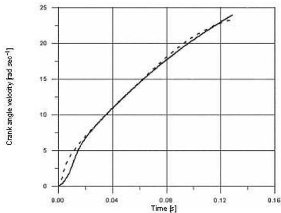
**Figure 7** Crank angle velocity versus time for FEM model ( - - - - ) and ADAMS model ( ——— )
