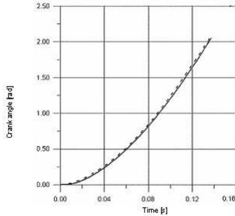
**Figure 6** Crank angle versus time for FEM model ( - - - - ) and ADAMS model ( ——— )
