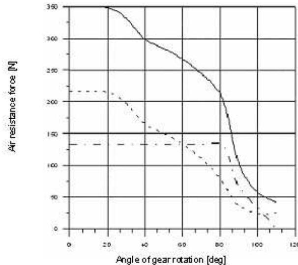
**Figure 3** Course of air resistance with angle of gear rotation: (—) resistance of the whole gear, (- - -) undercarriage leg, (- · - · -) wheel resistance
