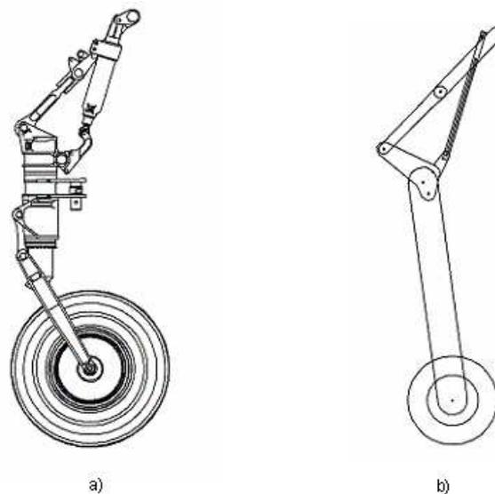
**Figure 1** Constructional model of landing gear (a) and its beam-type model (b)
