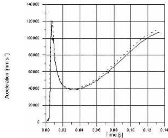
**Figure 11** Acceleration of kinematic pair 2 versus time with (—) and without (---) friction
