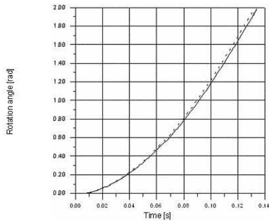
**Figure 9** Rotation angle of the crank versus time with (—) and without ( - - - ) friction
