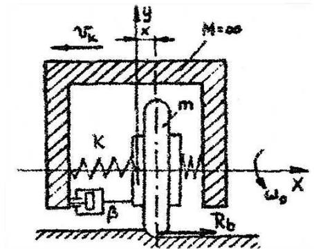
Figure 3 The vibrating system with 1 DOF
