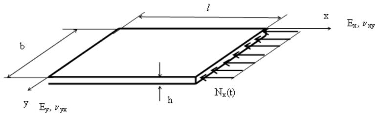
Figure 1 Geometry and loading of a plate
