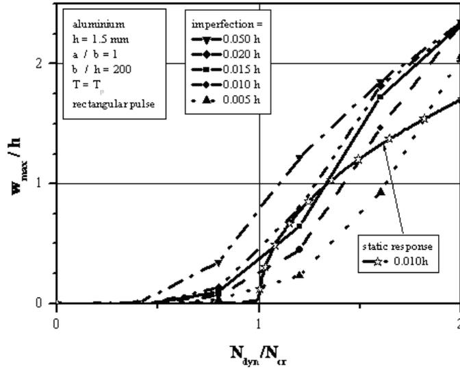
Figure 7 The dynamic response of a plate for a pulse loading for different values of geometric imperfection amplitudes and the static response
