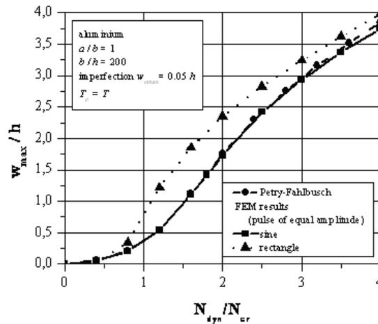
Figure 4 Comparison of the results obtained using ANSYS software and the results obtained by Petry and Fahlbusch
