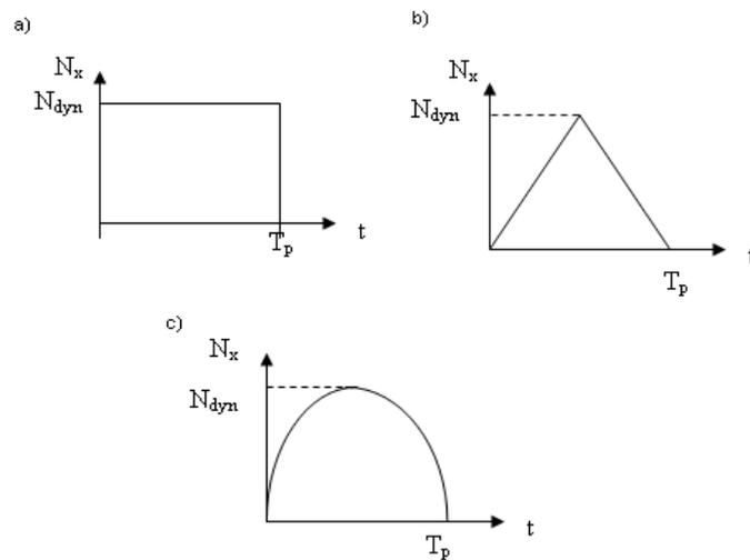
Figure 2 Shapes of pulse loading (in all cases for  $t > T_p \rightarrow N_x(t) = 0$ )
