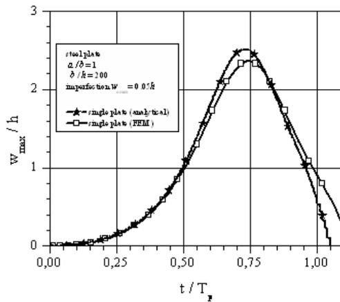
Figure 3 The response of a steel plate for rectangular pulse
