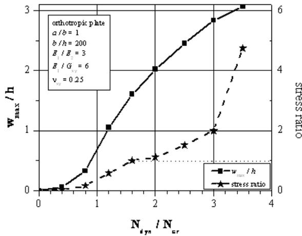
Figure 10 Maximal deflection and stress ratio versus amplitude of pulse loading
