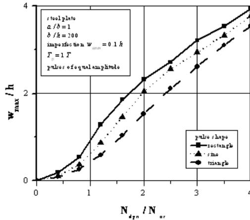
**Figure 5** Influence of a pulse shape on the maximal deflection of isotropic plate (pulses of equal amplitude)
