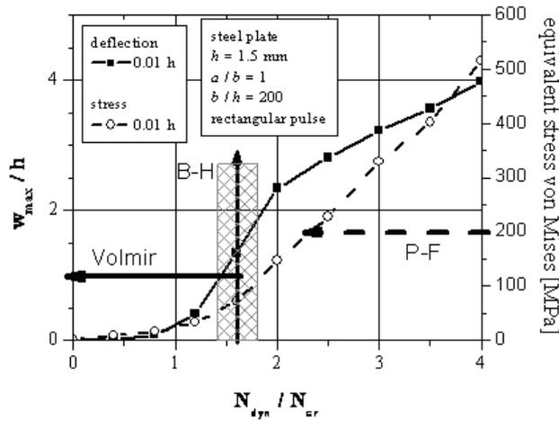
Figure 8 Estimation of DLF value according to assumed dynamic buckling criteria
