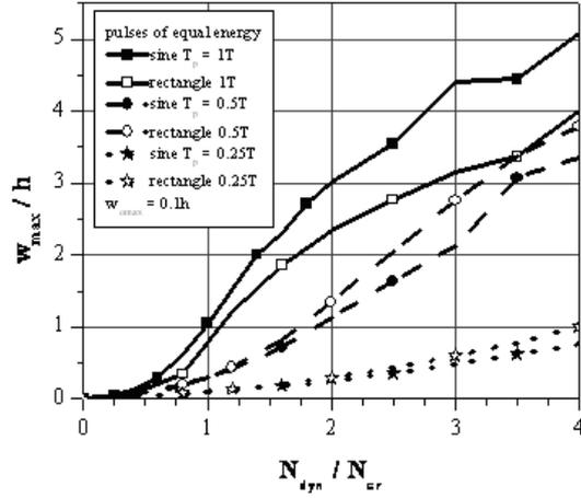
Figure 6 Influence of a pulse shape on the maximal deflection of isotropic steel plate ( $a/b=1$ ;  $b/h=200$ ) for different time of pulse duration (pulses of equal energy)
