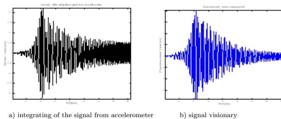
**Figure 5** Value component of the vertical movement along the y-axis derived from the system of video (b) and integration of signal from accelerometer (a) a) integrating the signal from accelerometer b) the differential video signal
