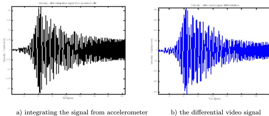
**Figure 6** Value component of the vertical speed along the y-axis obtained: after integration signal from accelerometer (a) and after shipment differentiation of signal obtained from the vision data (b)
