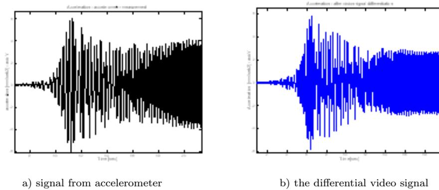
**Figure 4** Value component of the vertical velocity along the y-axis derived from accelerometer a) and from the video after a double movement signal after differentiation b)
