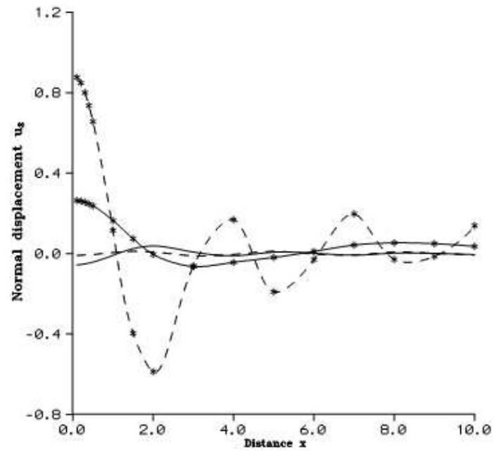
**Figure 4** Variation of Normal displacement  $u_2$  with horizontal distance  $x$  due to uniformly distributed force
