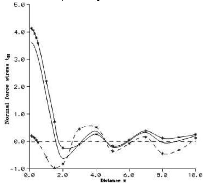
Figure 8 Variation of Normal force stress  $t_{22}$  with horizontal distance  $x$  due to a moving force
