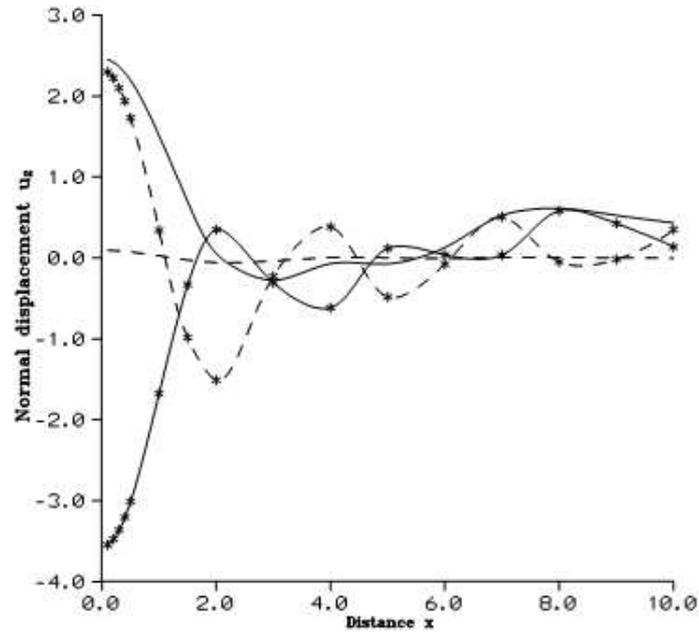
Figure 7 Variation of Normal displacement  $u_2$  with horizontal distance  $x$  due to a moving force
