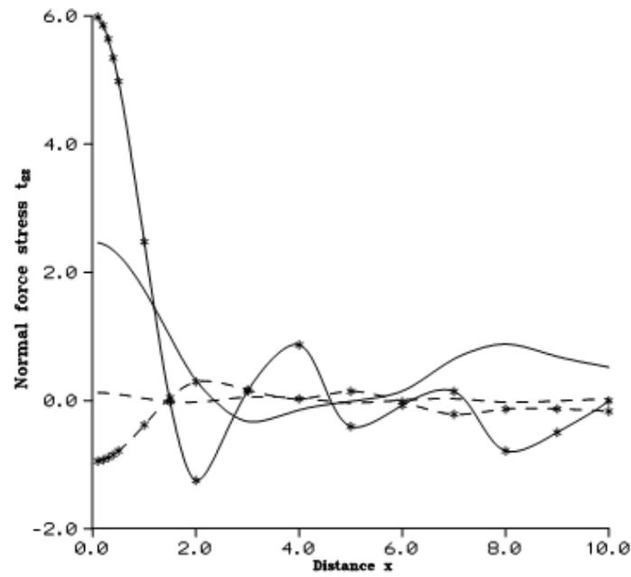
Figure 2 Variation of Normal force stress  $t_{22}$  with horizontal distance  $x$  due to concentrated force
