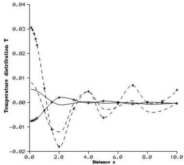
**Figure 3** Variation of Temperature distribution  $T$  with horizontal distance  $x$  due to concentrated force
