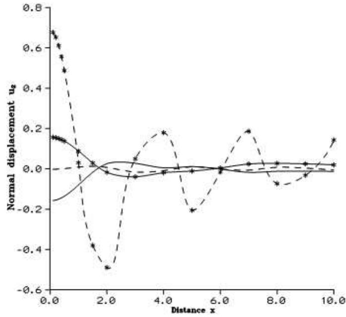
Figure 1 Variation of Normal displacement  $u_2$  with horizontal distance  $x$  due to concentrated force
