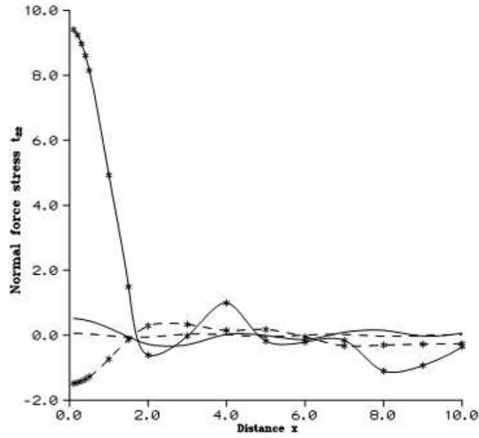
Figure 5 Variation of Normal force stress  $t_{22}$  with horizontal distance  $x$  due to uniformly distributed force
