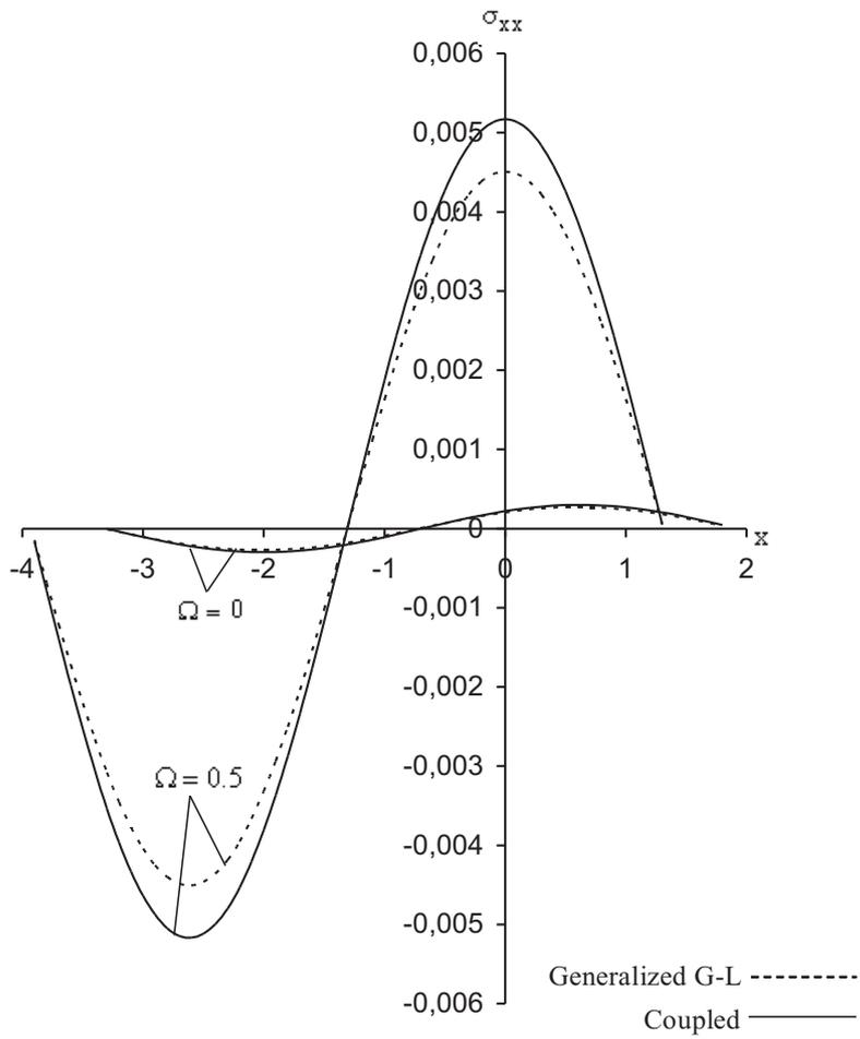
Figure 6 The distribution of stress component  $\sigma_{xx}$  on the surface at  $t = 1$ .
