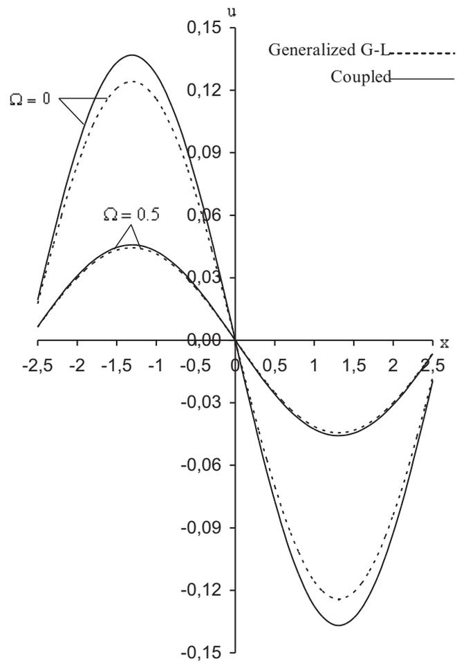
**Figure 9** Horizontal displacement distribution  $u$  on the middle plane at  $t = 1$ .
