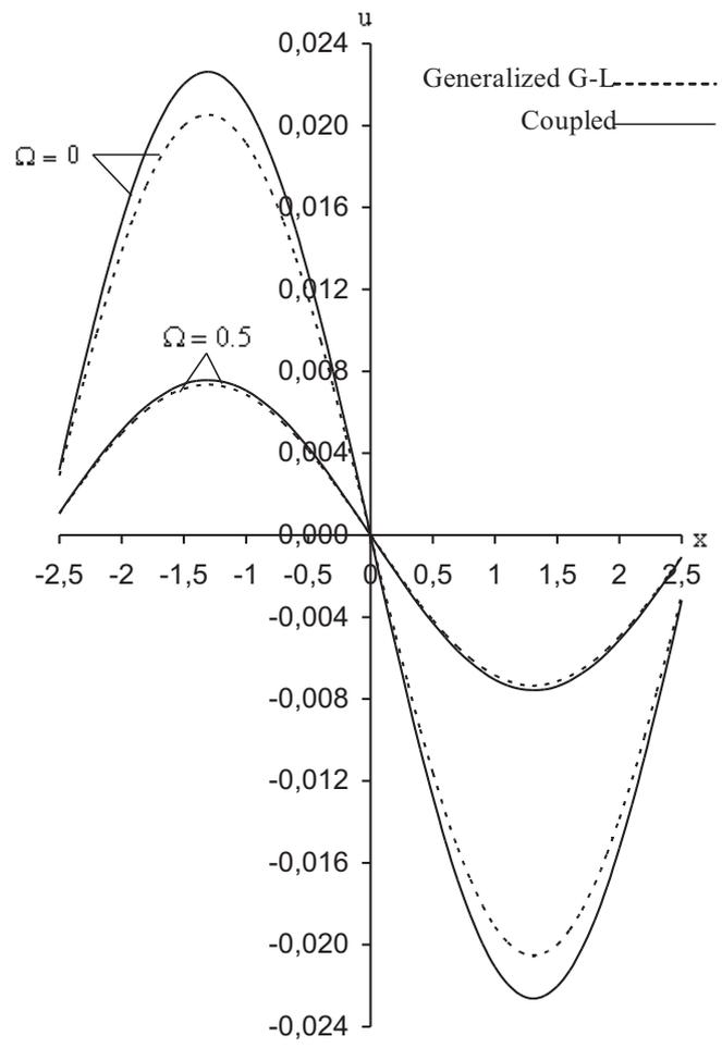
Figure 8 Horizontal displacement distribution u on the middle plane at  $t = 0.1$ .
