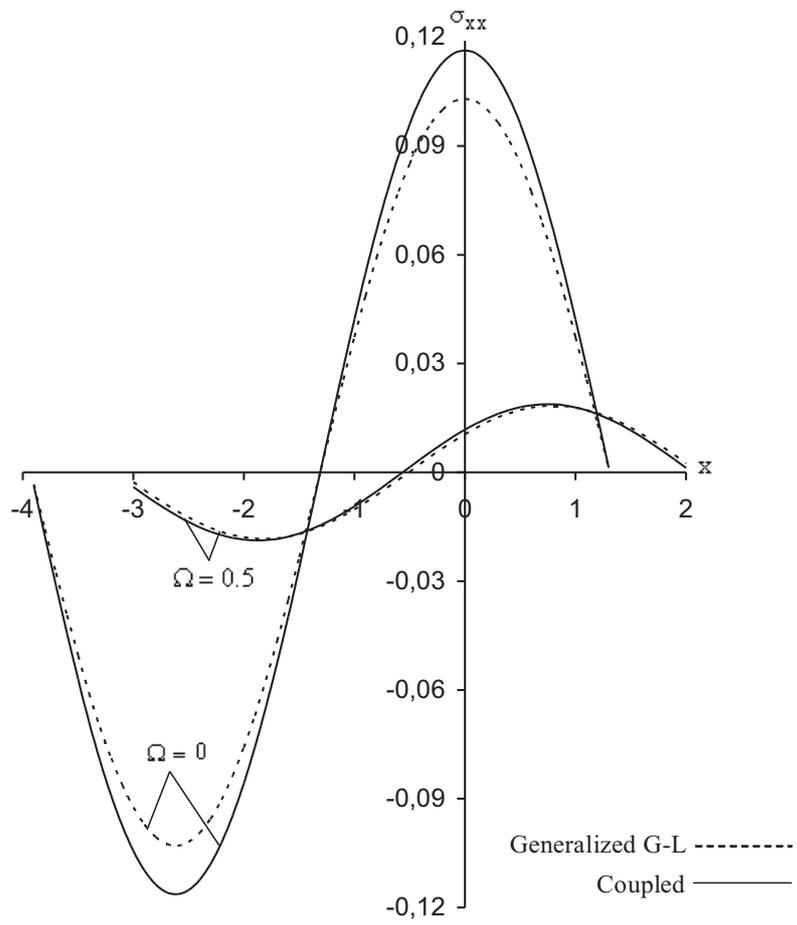
**Figure 11** The distribution of stress component  $\sigma_{xx}$  on the middle plane at  $t = 1$ .
