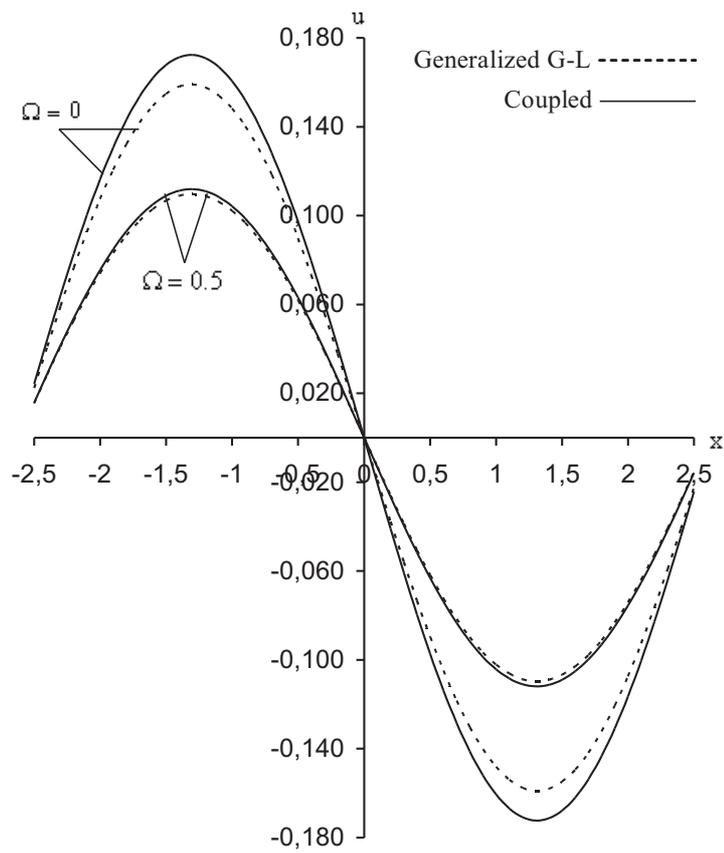
**Figure 3** Horizontal displacement distribution  $u$  on the surface at  $t = 0.1$ .
