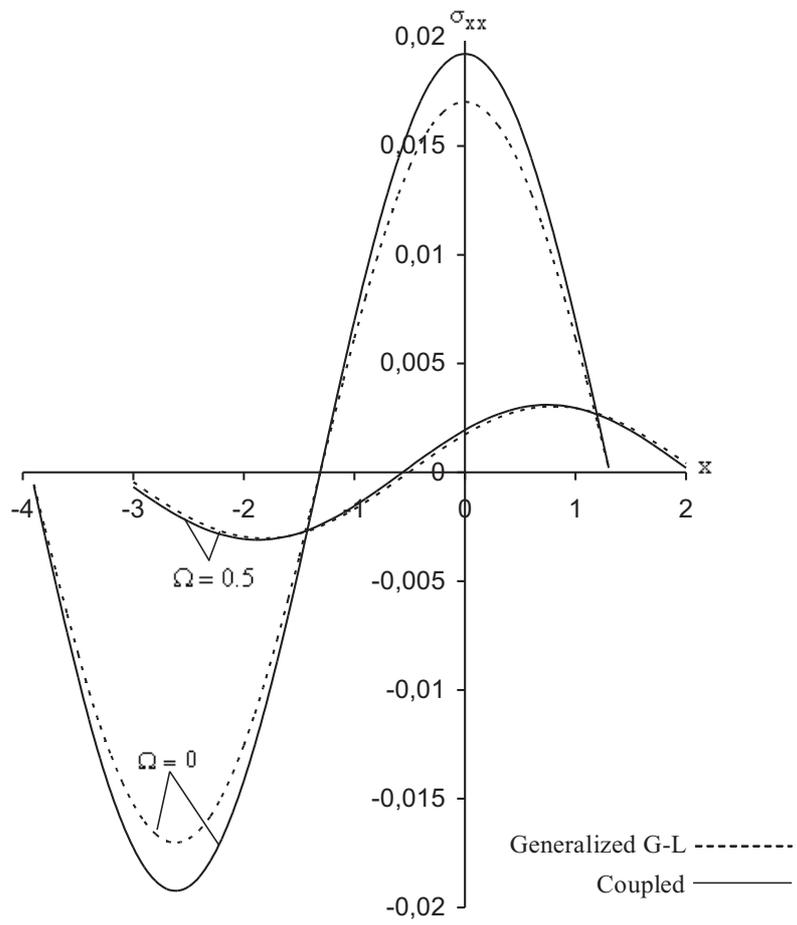
**Figure 10** The distribution of stress component  $\sigma_{xx}$  on the middle plane at  $t = 0.1$ .
