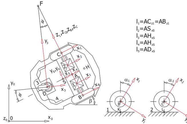
**Figure 1** Computation model of AmigoBot<sup>TM</sup> robot
