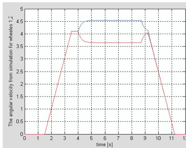
**Figure 3** The angular velocities time courses from simulation:  $\dot{\alpha}_1$  [rad/s]– blue,  $\dot{\alpha}_2$  [rad/s]– red
