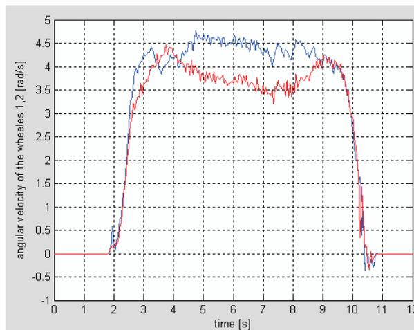
**Figure 5** The angular velocities time courses from test rig:  $\dot{\alpha}_1$  [rad/s] – blue,  $\dot{\alpha}_2$  [rad/s]– red
