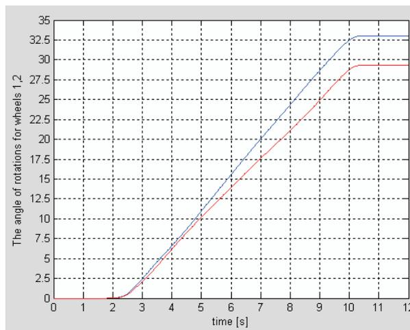
**Figure 4** The angles of rotations time courses from test rig:  $\alpha_1$  [rad] – blue,  $\alpha_2$  [rad]– red
