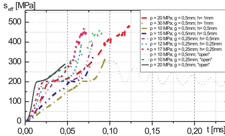
**Figure 5** Curves of the maximal effective stress in the whole structure versus time for different pressure amplitudes
