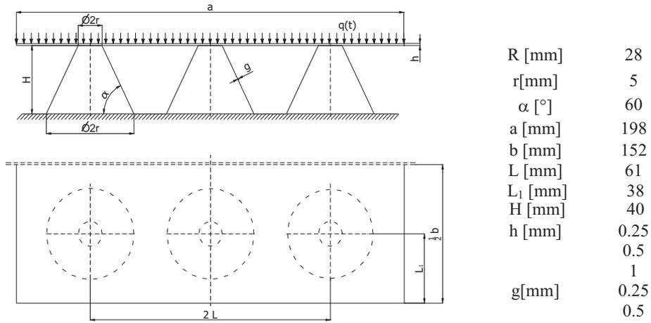
**Figure 1** Structure of the absorber – dimensions and the loading method
