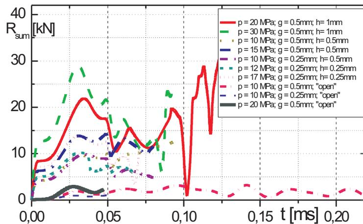
Figure 7 Curves of the ground reaction versus time for different pressure amplitudes
