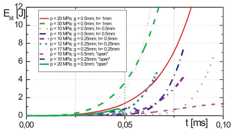
**Figure 8** Curves of the summary strain energy versus time for different pressure amplitudes
