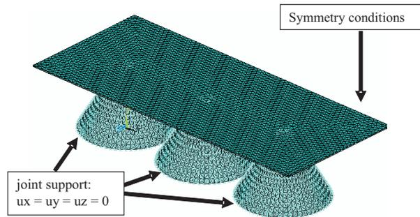
**Figure 4** Numerical model of the absorber in the ANSYS code
