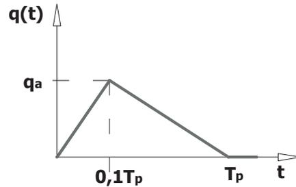
**Figure 2** Pressure pulse shape:  $q(t)$  – pressure,  $T_p$  – duration of the pulse,  $q_a$  – amplitude of pressure the pulse
