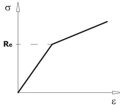
**Figure 3** Bilinear strain–stress curve of the ultimate strength:  $R_e$  – yield stress
