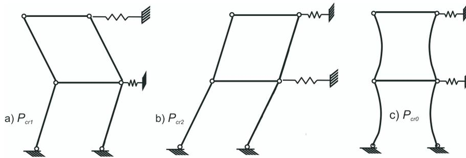
**Figure 3** Buckling modes corresponding to calculated buckling loads and to the maximal buckling load for Winter-type model of frame
