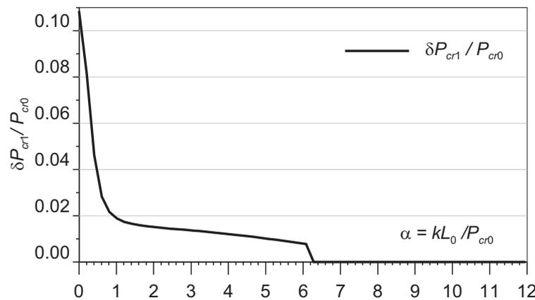
Figure 7 Relative variation of the first buckling load vs. bracing stiffness parameter  $\alpha$
