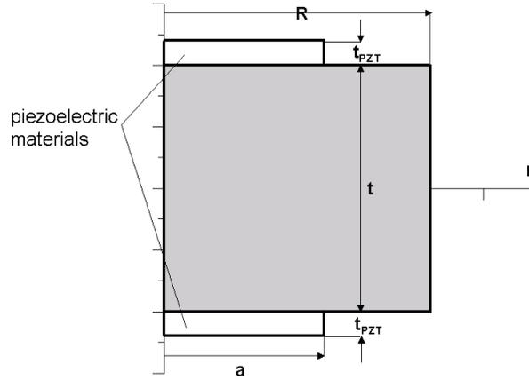
**Figure 1** Geometry of piezoelectric circular plate (cross-section)
