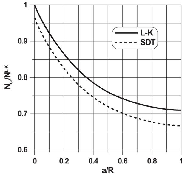
**Figure 2** Influence of width of piezoelectric layer on value of critical force (L-K – Love-Kirchhoff theory, SDT – first order shear deformation theory)
