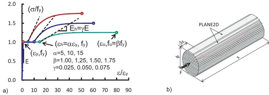
Figure 1 a) Parameters of mechanical properties of steel, b) Numerical model of a bar
