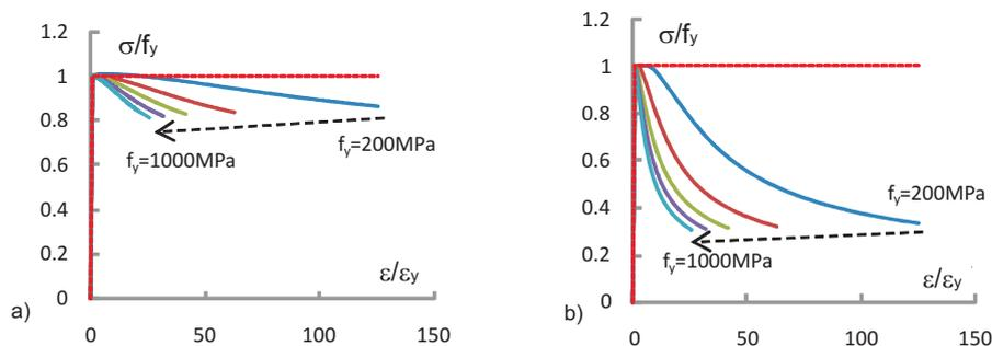
**Figure 2** The impact of yield strength on the equilibrium paths of bars of elasto-perfectly plastic characteristic: a) bar slenderness  $s/\phi=5$ , b) bar slenderness  $s/\phi = 10$
