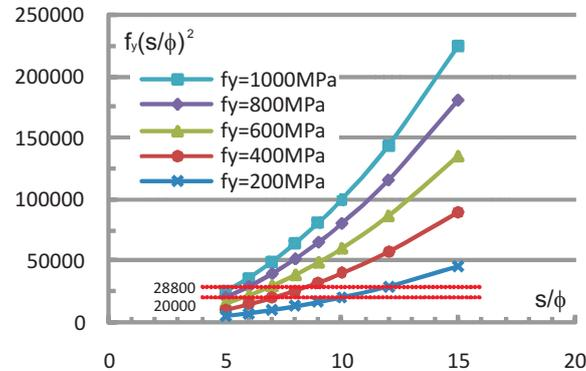
Figure 5 Graphs of relations  $f_y (s/\phi)^2$  for various yield strengths
