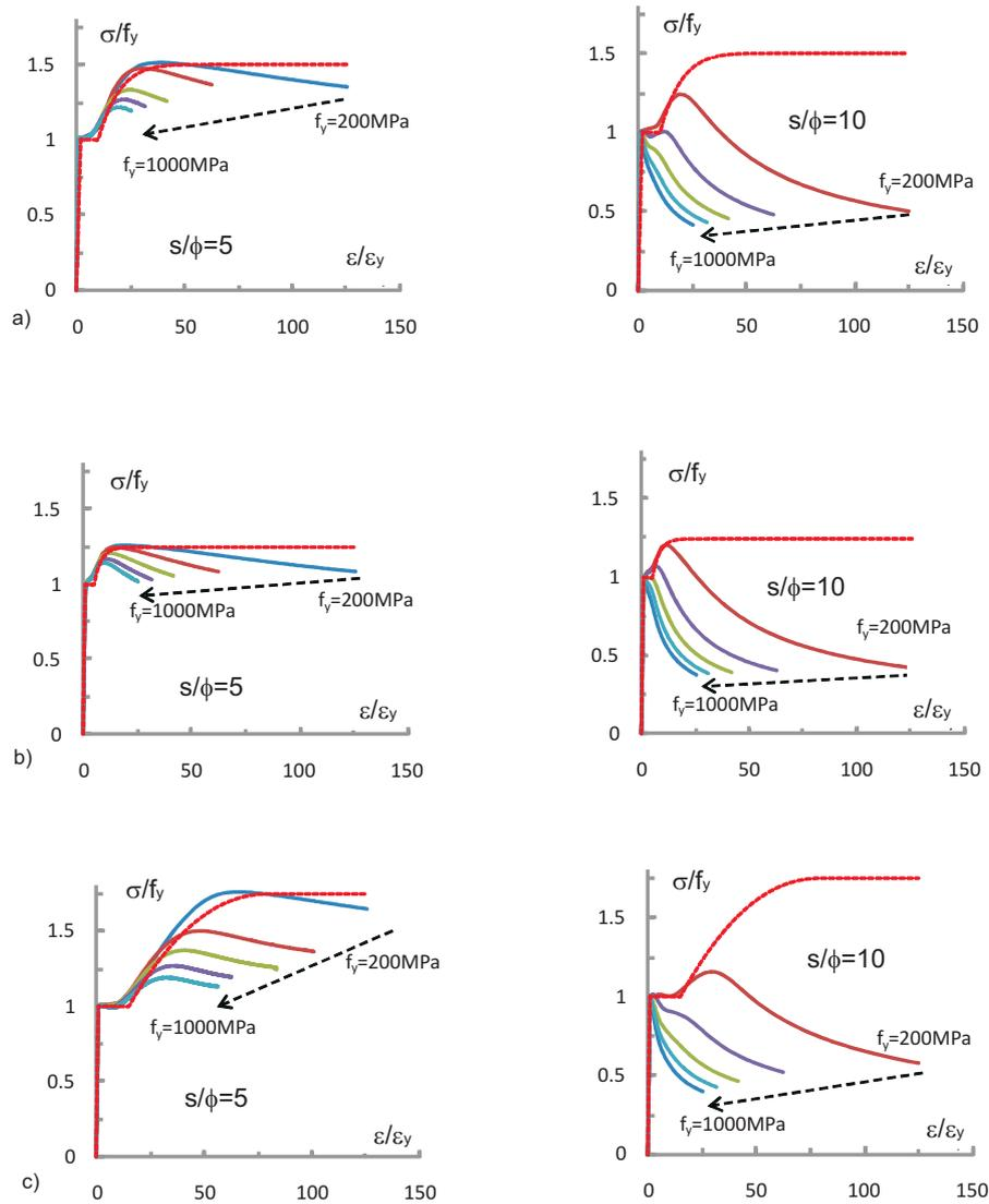
**Figure 3** Impact of yield strength on equilibrium paths of bars of elasto-plastic characteristic with strengthening: a) steel bars with steel parameters  $\alpha = 10$ ,  $\beta = 1.50$ ,  $\gamma = 0.050$ , b) steel bars with steel parameters  $\alpha = 5$ ,  $\beta = 1.25$ ,  $\gamma = 0.075$ , c) steel bars with steel parameters  $\alpha = 15$ ,  $\beta = 1.75$ ,  $\gamma = 0.025$
