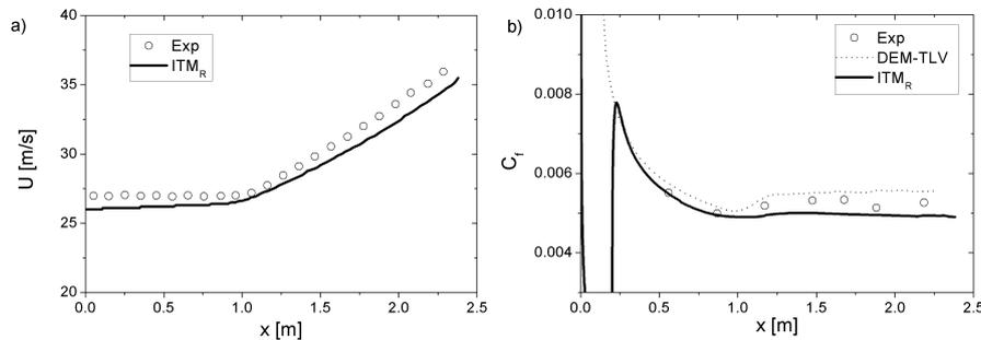
**Figure 3** Evolution of velocity  $U$  (a) and skin friction coefficient  $C_f$  (b) for non-zero pressure gradient test case ( $U_\infty = 26$  m/s)
