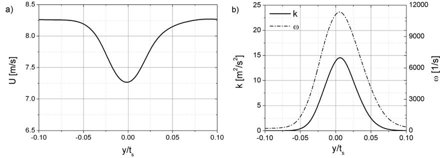
**Figure 1** Inlet profiles for unsteady calculations: velocity  $U$  (a) turbulent kinetic energy  $k$  and specific dissipation rate  $\omega$  (b)
