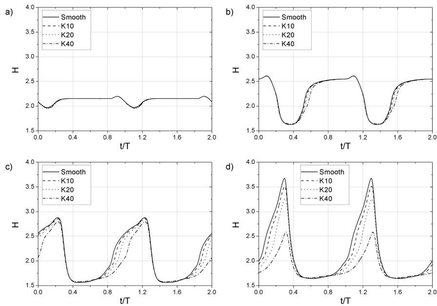
**Figure 7** Time traces of shape factor  $H$  at the location  $S_s=0.3$  (a)  $S_s=0.65$  (b)  $S_s=0.85$  (c)  $S_s=0.95$  (d)
