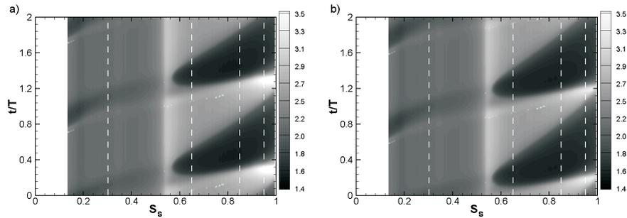
**Figure 6** S-t diagrams of shape factor  $H$  over the suction side for test cases: smooth surface (a) with roughness - K20 (b)
