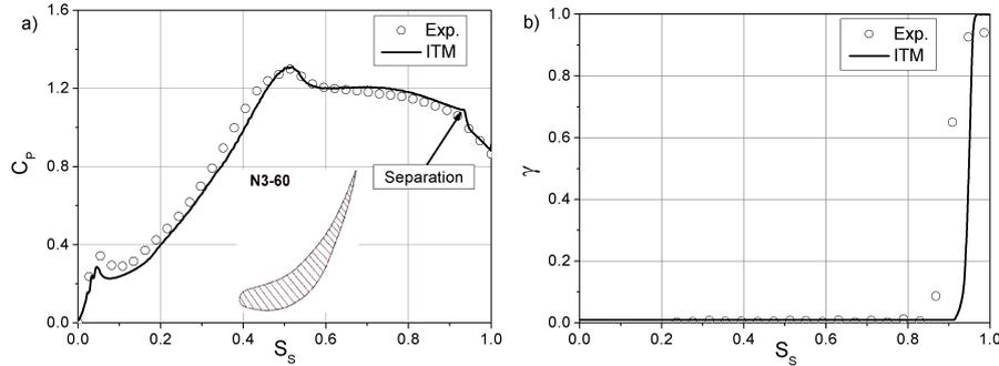
**Figure 4** Evolution of pressure coefficient  $C_p$  (a) and intermittency  $\gamma$  (b) for the N3-60 test case ( $Tu = 0.4\%$ )
