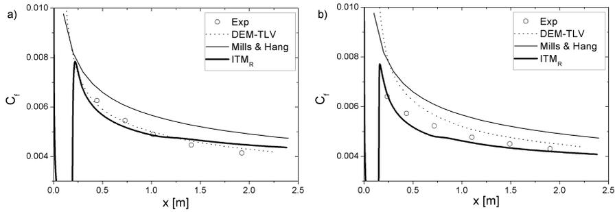
**Figure 2** Skin friction coefficient  $C_f$  for zero-pressure gradient test case:  $U_\infty = 27$  m/s (a)  $U_\infty = 42$  m/s (b)
