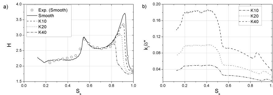
**Figure 5** Shape factor  $H$  (a) and  $k_r/\delta^*$  (b) for the N3-60 test case ( $Tu = 0.4\%$ )
