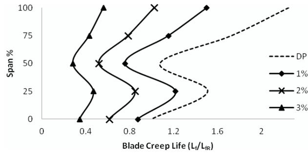
Figure 8 Blade creep life for compressor degradation at  $T_{amb}$  288.15 K
