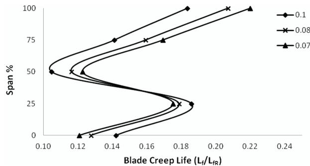
**Figure 5** Blade creep life ( $L_f/L_r$ ) along blade span at TET 1540 K and  $T_{amb}$  318.15 K
