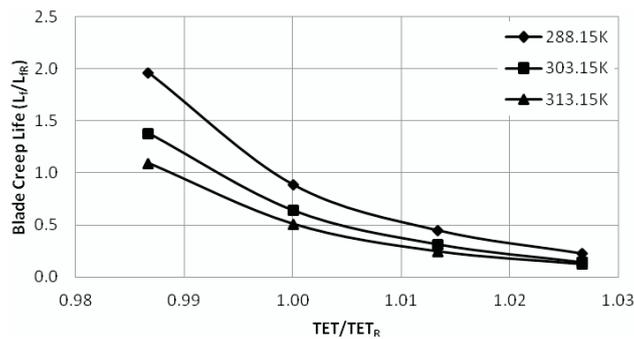
Figure 7 Blade creep life at different  $T_{amb}$  for RTDF 0.08
