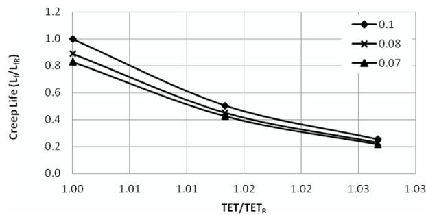
Figure 6 Blade creep life at the root for different RTDF at  $T_{amb}$  288.15 K
