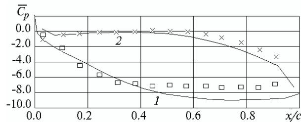
**Figure 2** The time averaged pressure coefficient distribution over the blade chord (1 suction side, 2 pressure side, [ ] pressure side experiment,  $\times$  suction side experiment)
