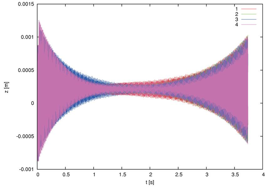
**Figure 4** Bending blade motion with 150 Hz excitation frequency and +90 deg phase angle in long time response
