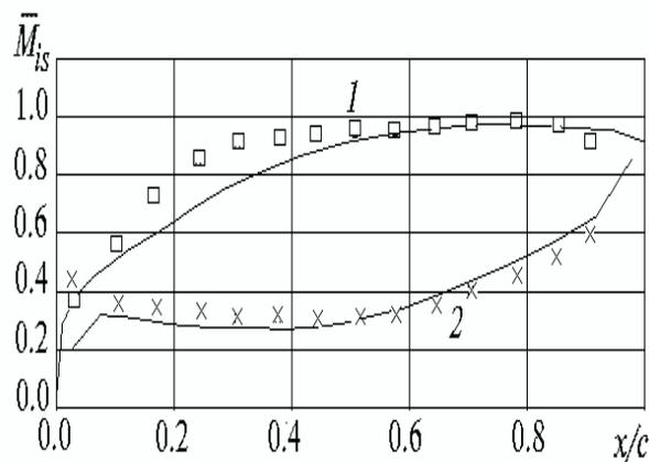
**Figure 3** The Mach number (b) distribution over the blade chord (1 suction side, 2 pressure side, [ ] pressure side experiment,  $\times$  suction side experiment)
