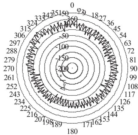
**Figure 3** Exemplary variation of a worm gear kinematic deviation in a function of a worm - wheel rotation angle  $\varphi_2$  presented in a radar graph
