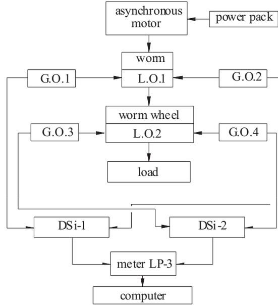
**Figure 5** Scheme of a worm gear's kinematic deviation measuring system
