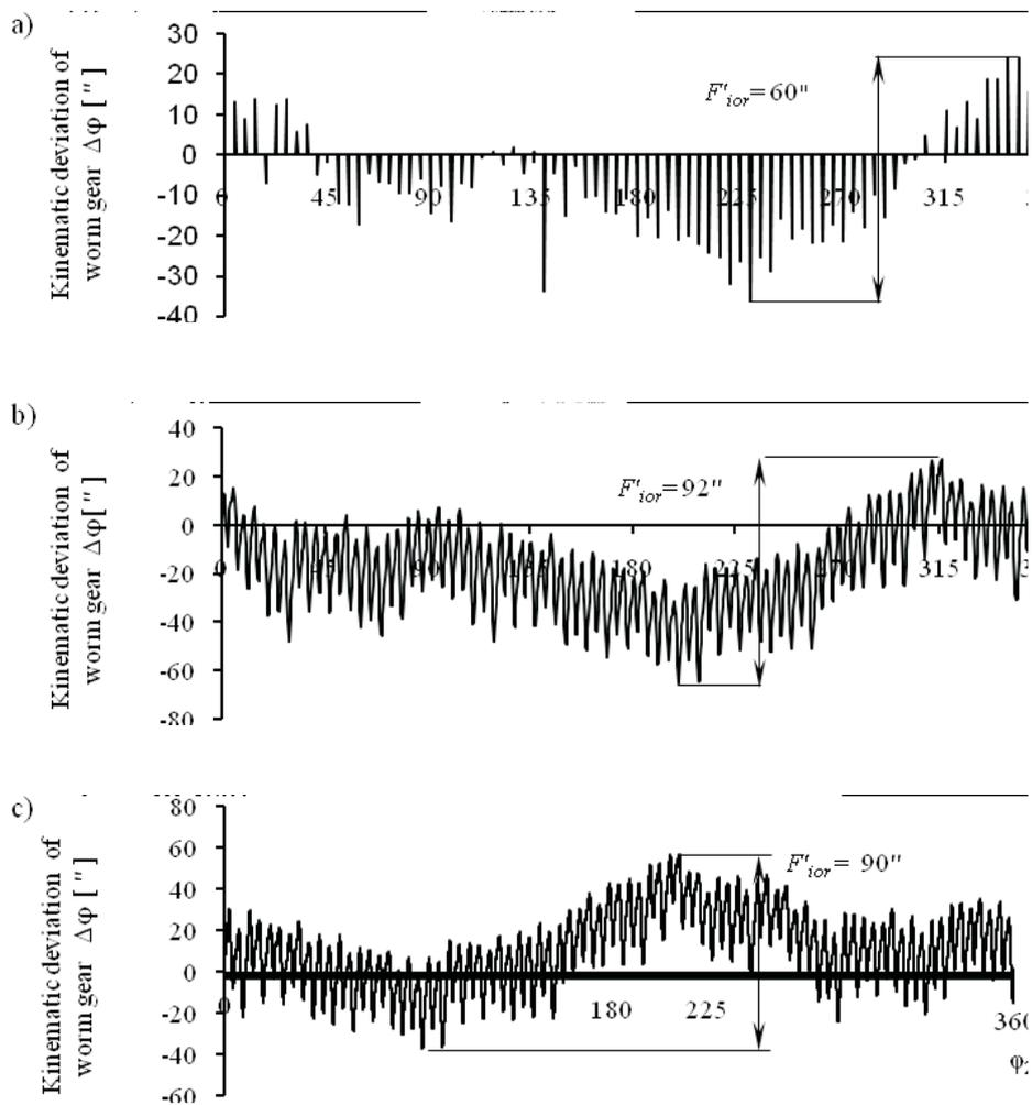
**Figure 6** Exemplary results of kinematic deviation measurement  $\Delta\varphi$  of a gear A80 in function of worm wheel's rotation angle  $\varphi_2$  for measuring step : a)  $L_1 = 360^\circ$ , b)  $L_1 = 30^\circ$ , c)  $L_1 = 1^\circ$
