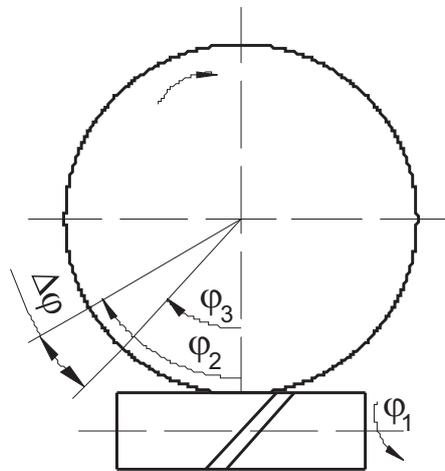
**Figure 1** Kinematic deviation of worm gear
