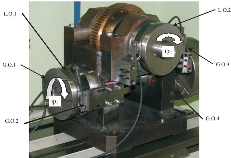
**Figure 4** A gear A80 with assembled measuring system of rotation angle
