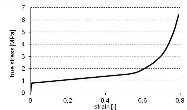
**Figure 5** Material stress–strain relation obtained in laboratory for aluminum foam in compression test
