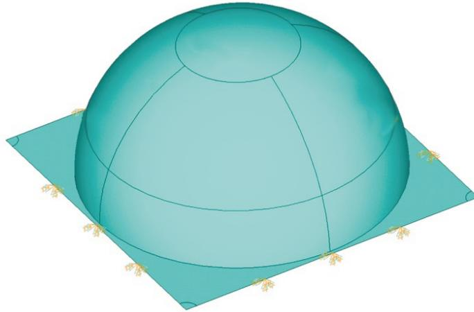
**Figure 3** Boundary conditions of analysed hemispherical shell
