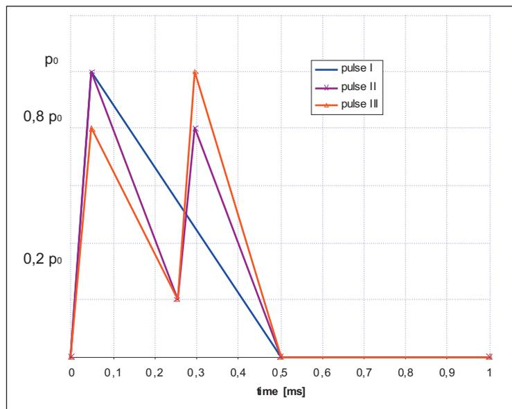
Figure 2 Assumed simulations of reflected blast pressure [4]
