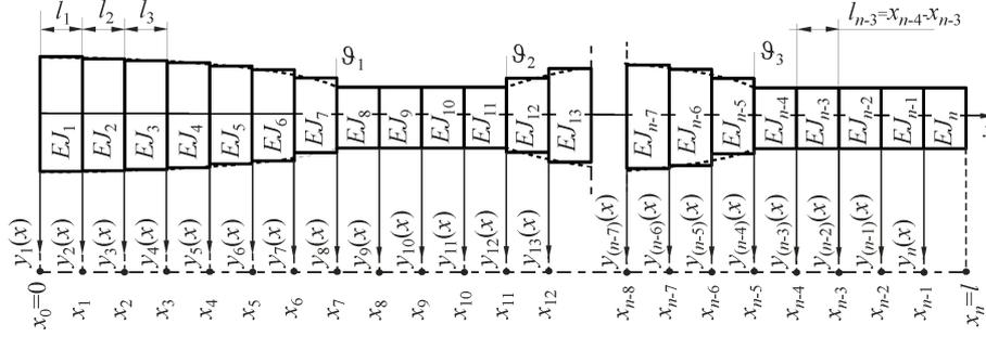
**Figure 3** Division of the optimised column into prismatic segments (system  $\text{COr}(R^*)$ )
