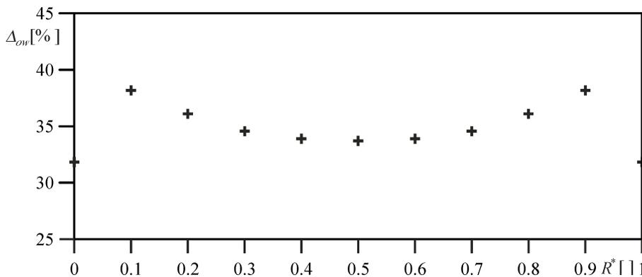
**Figure 5** Percentage increase of the critical load  $\Delta_{ow}$  with regard to the head parameter  $R^*$  values of the system  $COr(R^*)$  for  $\chi = 3$
