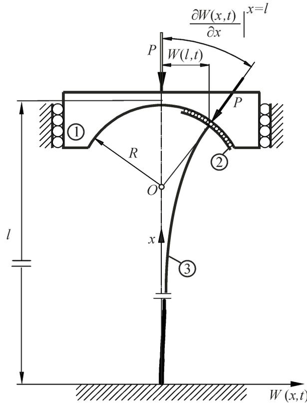
**Figure 1** The physical model of the column loaded by the follower force directed towards the positive pole (comp. [2, 3, 4])
