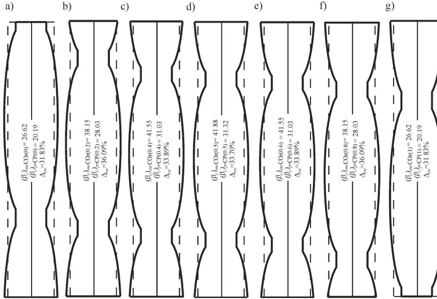
**Figure 6** Optimal shapes of columns which fulfils strength condition (14) with regard to value of parameter  $R^*$  of the system  $\text{COr}(R^*)$  for  $\chi = 3$
