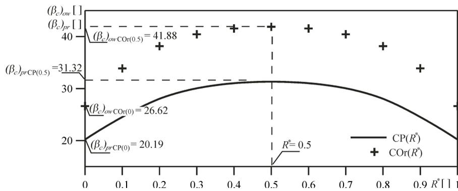
**Figure 4** Critical load parameters  $(\beta_c)_{ow}$  and  $(\beta_c)_{pr}$  change depending on the head parameter  $R^*$  of the systems  $COr(R^*)$  for  $\chi = 3$  and  $CP(R^*)$
