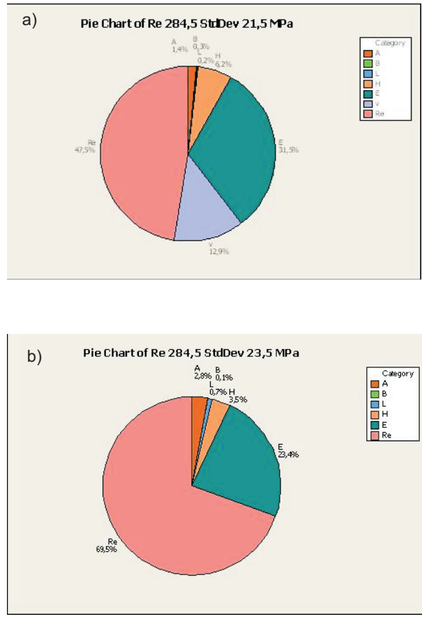
Figure 4 Exemplary pie charts (UBELC sensitivity analysis – yield stress variance): a) – 21.5 MPa standard deviation, b) – 23.5 MPa standard deviation
