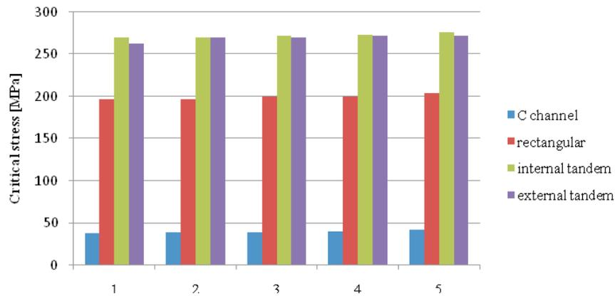
Figure 5 First 5 lowest values of critical stress for the axially compressed beams of different cross-sections
