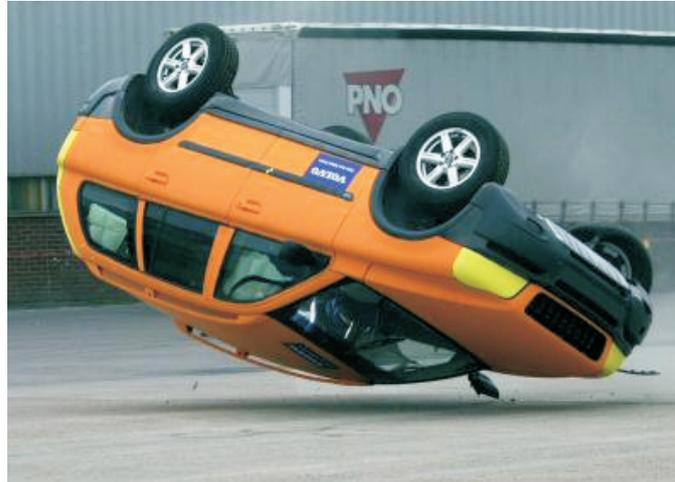
**Figure 9** Rollover crash test of Volvo XC90 [7]
