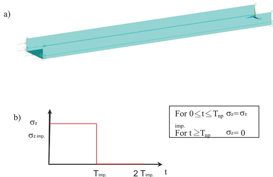
**Figure 3** Loading details: a) C channel boundary conditions, b) The rectangular impulse loading characteristics
