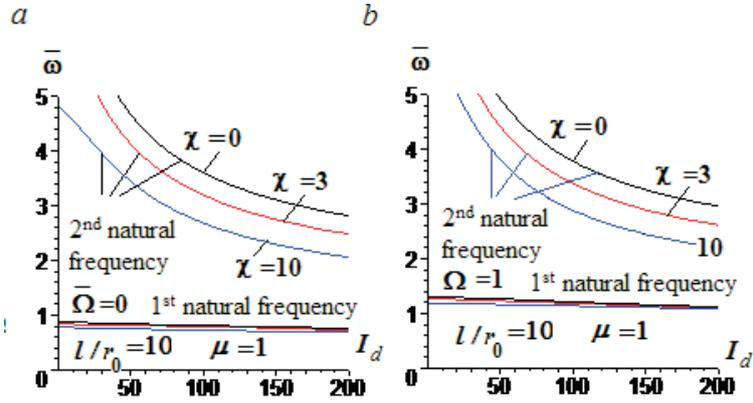
Figure 9 The normalized frequency  $\bar{\omega}$  via the normalized moment of inertia of the end mass at  $l/r_0=10$ ;  $\mu = 1$ , with different value; (a)  $\bar{\Omega} = 0$ , (b) the angular velocity  $\bar{\Omega} = 1$
