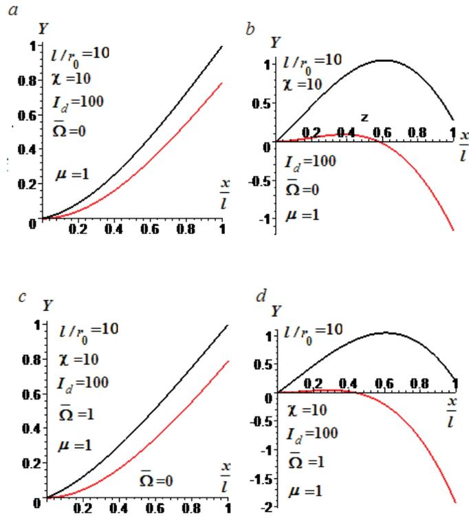
Figure 10 The first and second natural shapes and the flexural components for a non-rotating (a, b) and rotating ( $\bar{\Omega} = 1$ ) beam (c, d) with  $I_d^*=100$  ( $l/r_0=10$ ,  $\mu = 1$ ,  $\chi=10$ )
