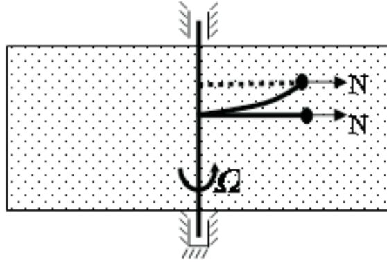
**Figure 1** A rotating cantilever beam with end mass
