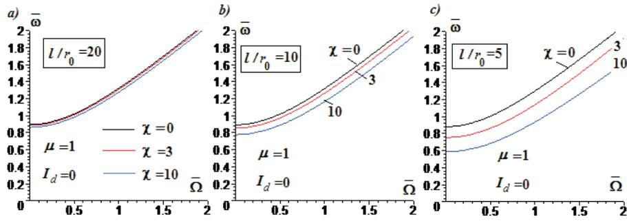
**Figure 3** Normalized first natural frequency via the normalized angular velocity for three values of the shear parameter  $\chi = 0, 3, 10$ : a)  $l/r_0 = 20$ ; b)  $l/r_0 = 10$ ; c)  $l/r_0 = 5$  ( $\mu = 1, I_d^* = 0$ )
