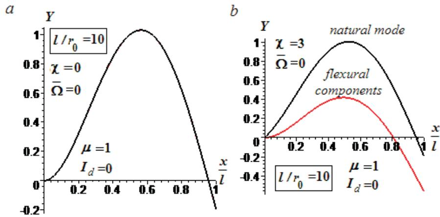
**Figure 6** The second natural mode of non-rotating beam  $l/r_0=10$ ;  $\mu=1$ ,  $J_d^*=0$ : a)  $\chi=0$ , b)  $\chi=3$
