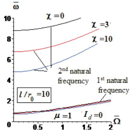
**Figure 5** The first and second normalized eigenfrequency  $\bar{\omega}_0$  via the angular velocity of rotation at  $l/r_0=10$ ;  $\mu=1$ ,  $J_d^*=0$ , for different  $\chi$ -values ( $\chi=0$ ; 3 and 10)
