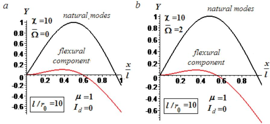
**Figure 7** The second natural modes of the beam with high shear deformability ( $\chi=10$  (a)  $\bar{\Omega} = 0$ ; (b)  $\bar{\Omega} = 2$  ( $l/r_0=10$ ;  $\mu = 1$ ,  $I_d^*=0$ ))
