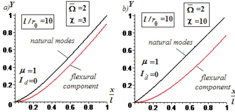
**Figure 4** The first natural modes and their flexural components for the beam  $l/r_0=10$ ,  $\mu = 1$ ,  $I_d^*=0$   $\bar{\Omega} = 2$  at two  $\chi$ - values:  $\chi=3$  (a) and  $\chi=10$  (b)
