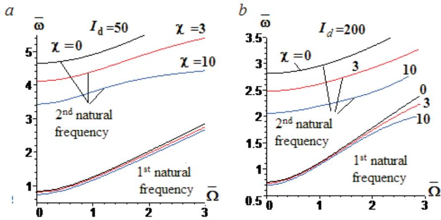
**Figure 8** Normalized first and second natural frequency  $\bar{\omega}$  via the normalized angular velocity for three  $\chi$  values at  $I_d^*=50$  (a) and  $I_d^*=200$ (b); ( $l/r_0=10$ ;  $\mu = 1$ )
