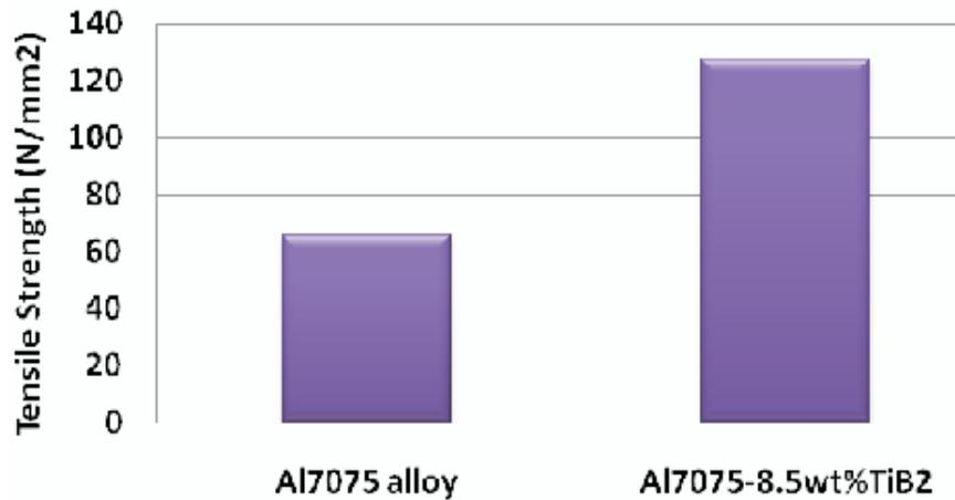
**Figure 4** Tensile Strength of Al7075 alloy and Al7075-TiB<sub>2</sub> composite
