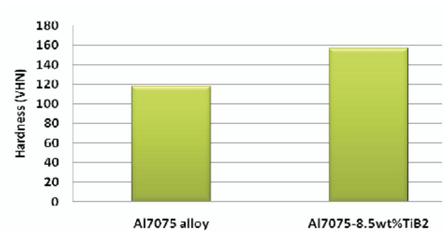
**Figure 3** Hardness of Al7075 alloy and Al7075-TiB<sub>2</sub> composite
