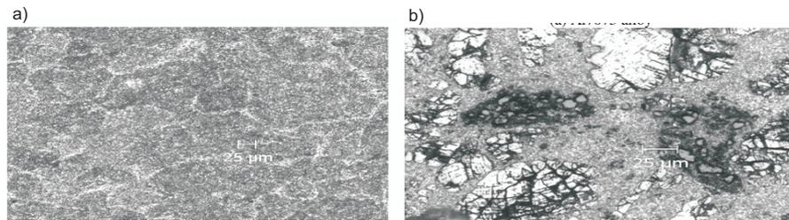
**Figure 2** Optical micro photographs of a) Al7075 alloy and b) Al7075 8.5wt% TiB<sub>2</sub> composite
