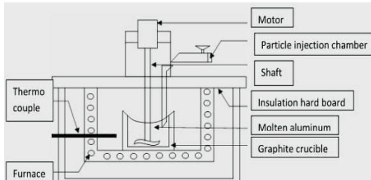
Figure 1 Stir casting Experimental set up
