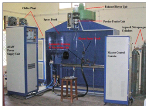
Figure 2 Experimental setup of atmospheric plasma spray process
