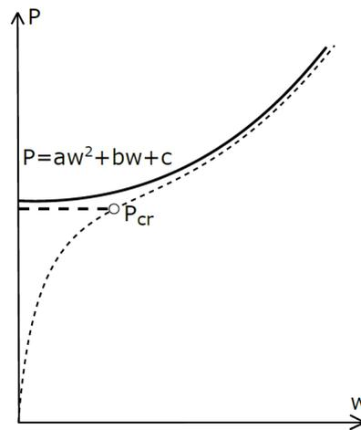
**Figure 4** Determining critical load using Koiter's method [24] – the behavior of ideal structure is represented by continuous line, the real by dotted one
