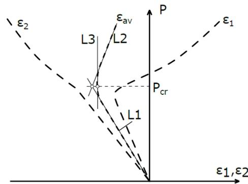
**Figure 6** Strains ( $\varepsilon_1$  and  $\varepsilon_2$ ), averaged strain ( $\varepsilon_{av}$ ) curves and methodology of finding critical load using averaged strain method (lines L1 and L2) and vertical tangent method (line L3) [24]
