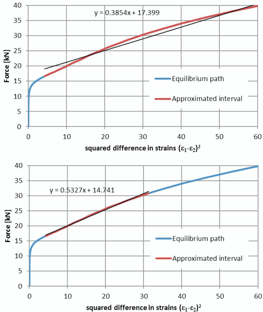
**Figure 11** a) and b) Plots representing the same equilibrium path on the load - squared difference in strains diagram with different linear approximations of post-buckling ranges
