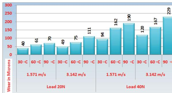
**Figure 3** Effect of temperature, load and sliding velocity on wear of AA 7075 – SiC composite
