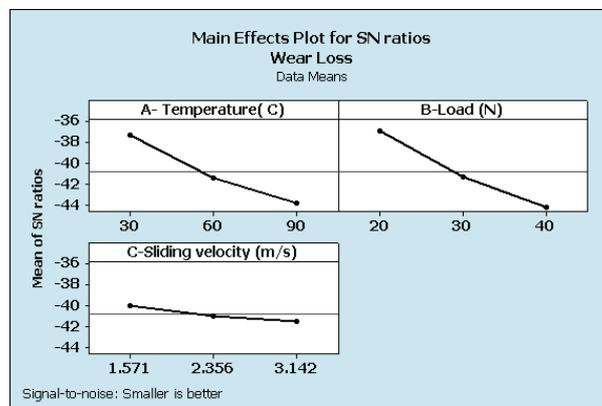
**Figure 5** The main effects plot for S/N ratio
