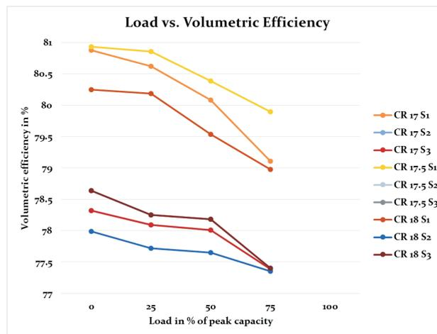
Figure 5 Response values of volumetric efficiency at various loads for each sample
