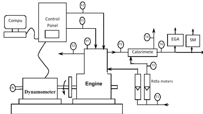
**Figure 1** Layout of the engine set up
