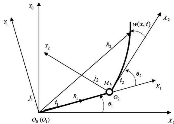
Figure 1 The schematic diagram of a two-link rigid-flexible manipulator
