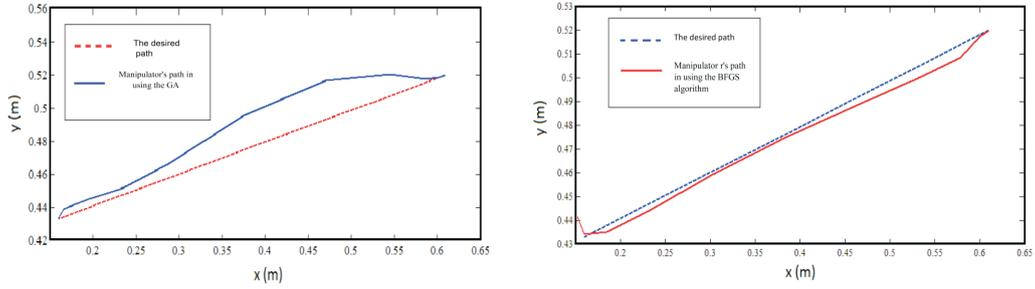
**Figure 4** Comparison between the traveled path by the manipulator and the desired path using the BFGS and the genetic algorithms
