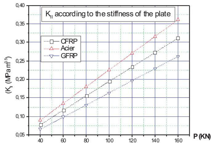
**Figure 11** Stress Intensity factor  $K_{II}$  in repaired beam based on the stiffness of the plate (where  $L_p = 2400$  mm, thickness  $t = 4$  mm)
