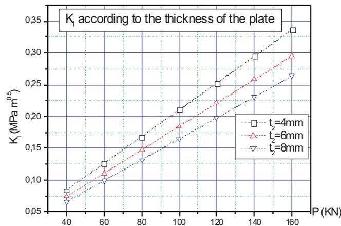
**Figure 6** Stress Intensity factor  $K_I$  in repaired beams according to the thickness of the plate for a length of strengthening  $L_p = 2400 \text{ mm}$
