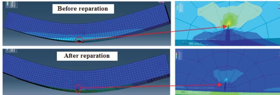
Figure 4 Effect of CFRP on the behaviour of cracked beams
