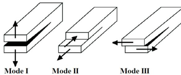
Figure 2 Three basic modes of fracture propagation
