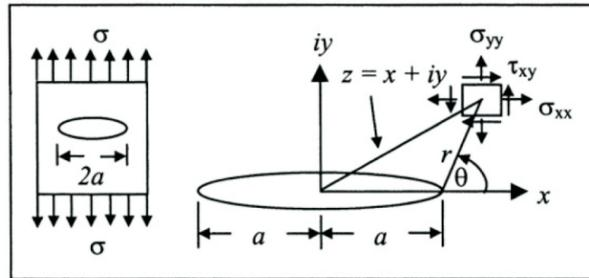
Figure 1 The crack tip stress field in complex coordinates
