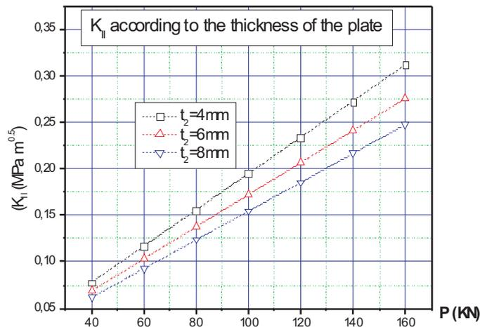
**Figure 9** Stress Intensity factor  $K_{II}$  in repaired beams according to the thickness of the plate for a length of strengthening  $L_p = 2400$  mm
