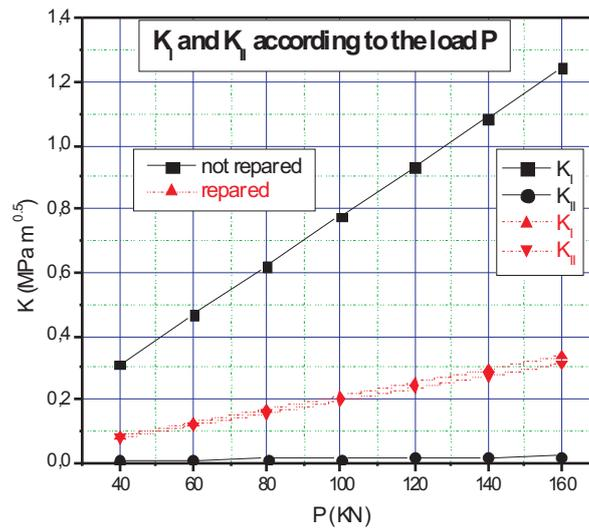
Figure 5 Propagation of cracks in notched beam before and after reparation
