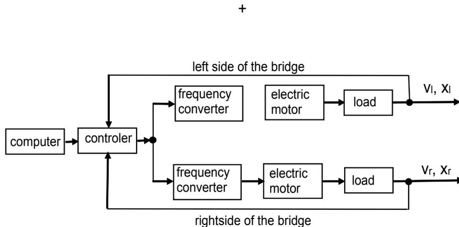
**Figure 3** A scheme of supplying and controlling motors of end-carriages of an overhead crane bridge
