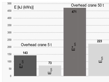
Figure 6 Energy profits  $E_{cn}$  in a norm cycle in comparison to the energy use  $E^*_{cn}$  of the drives without frequency converters
