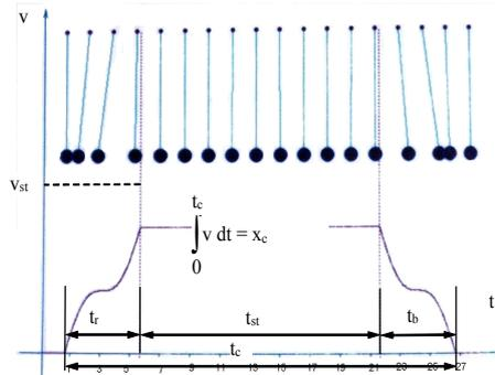
**Figure 1** Damping of load oscillation after starting and braking
