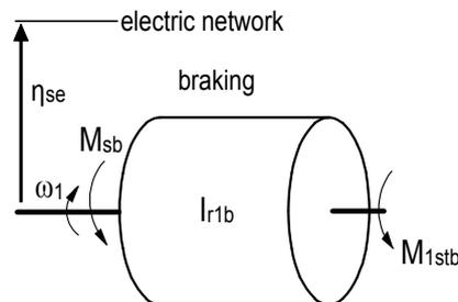
**Figure 2** A physical model of electric braking of the system of an overhead crane travelling
