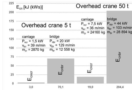
Figure 5 Energy profits in a norm cycle of overhead cranes
