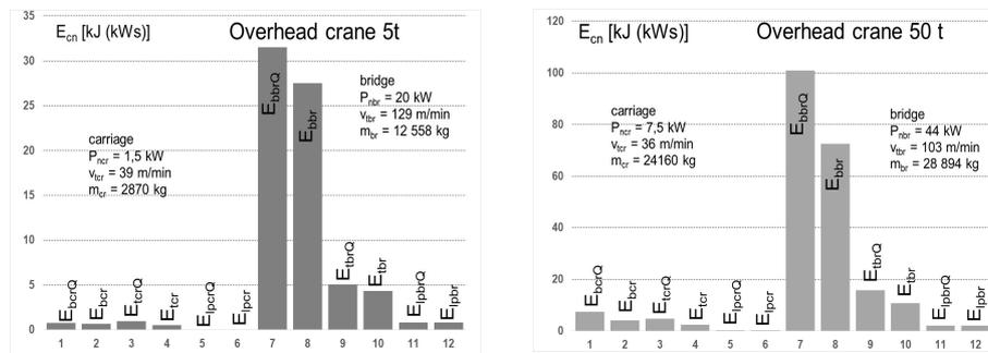
Figure 4 Distribution components of the energy profits in a norm cycle of overhead cranes
