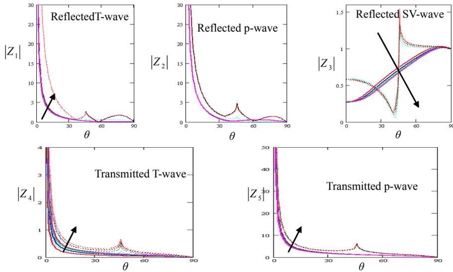
**Figure 9** Variation of the amplitudes  $z_i$  ( $i = 1, 2, \dots, 5$ ) with the angle of incidence of SV-wave for variation of magnetic field:  $H = 0.1, 0.2, 0.3, 0.4$ ,  $P = 1.1(10)^{11}$  (—),  $P = 0$  (...)
