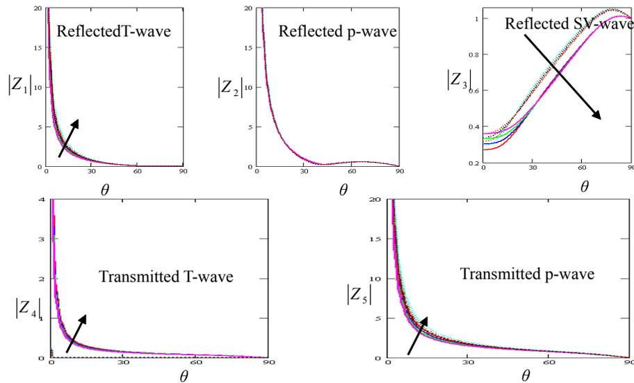
**Figure 11** Variation of the amplitudes  $z_i$  ( $i = 1, 2, \dots, 5$ ) with respect to  $(\theta, H)$  of SV-wave with and without variation of initial stress
