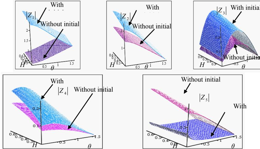
**Figure 8** Variation of the amplitudes  $z_i$  ( $i = 1, 2, \dots, 5$ ) with respect to  $(\theta, H)$  of thermal-wave with and without variation of initial stress
