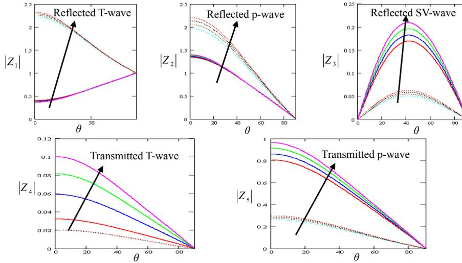
**Figure 6** Variation of the amplitudes  $z_i$  ( $i = 1, 2, \dots, 5$ ) with the angle of incidence of thermal-wave for variation of magnetic field:  $H = 0.1, 0.2, 0.3, 0.4$ ,  $P = 1.1(10)^{11}$  (—),  $P = 0$  (…)
