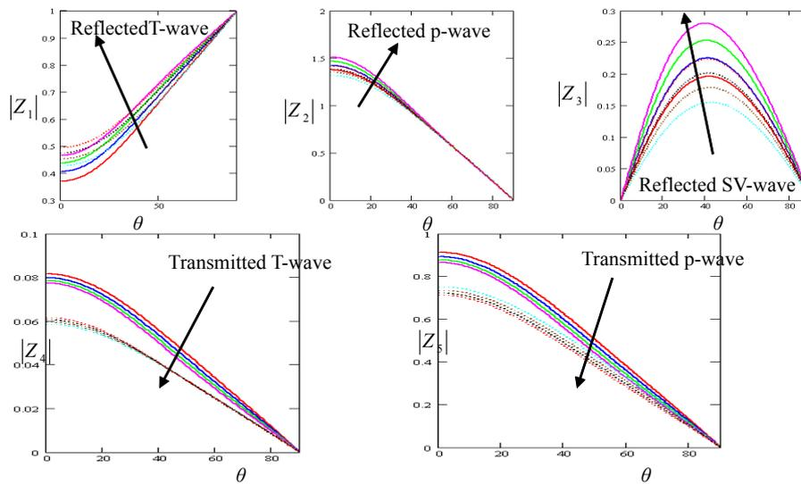
**Figure 7** Variation of the amplitudes  $z_i$  ( $i = 1, 2, \dots, 5$ ) with the angle of incidence of thermal-wave for variation of initial stress:  $P = (1.1, 1.2, 1.3, 1.4) (10)^{11}$ ,  $H = 0.3$  (—),  $H = 0$  (…)
