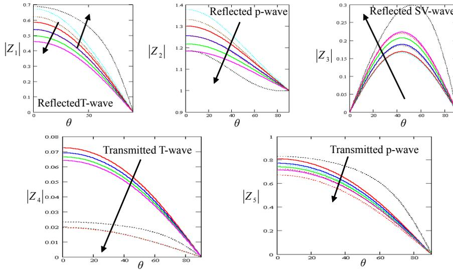
**Figure 3** Variation of the amplitudes  $z_i$  ( $i=1, 2, 5$ ) with the angle of incidence of p-wave for variation of magnetic field:  $H = 0.1, 0.2, 0.3, 0.4, P = 1.1(10)^{11}$  (—),  $P = 0$  (...)
