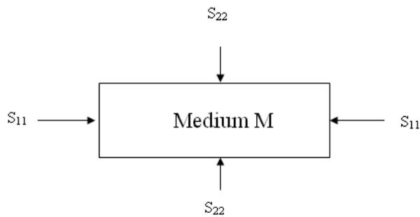
Figure 2 Components of initial stress in solid medium
