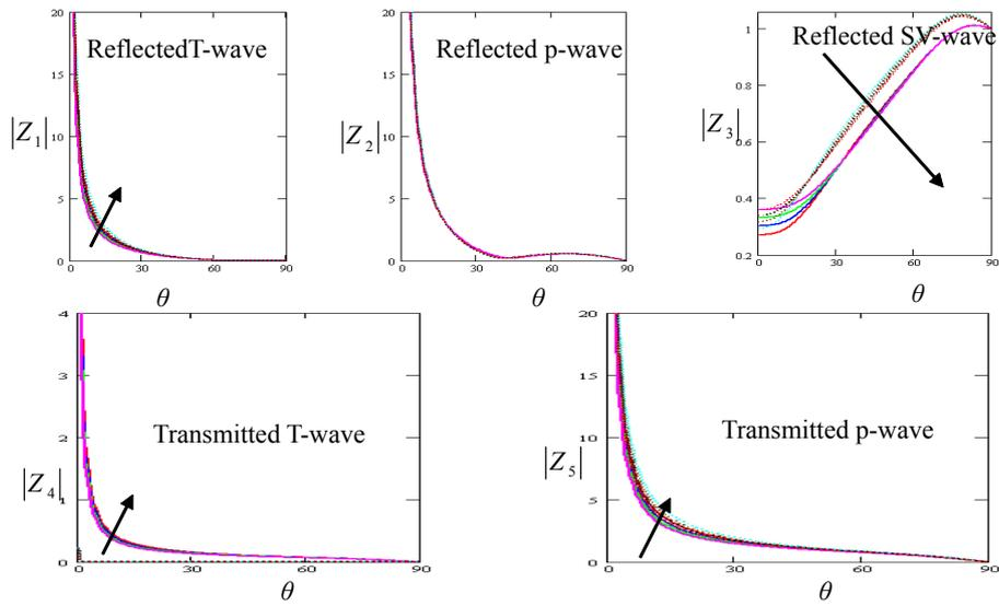
**Figure 10** Variation of the amplitudes  $z_i$  ( $i = 1, 2, \dots, 5$ ) with the angle of incidence of SV-wave for variation of initial stress:  $P = (1.1, 1.2, 1.3, 1.4) (10)^{11}$ ,  $H = 0.3$  (—),  $H = 0$  (...)
