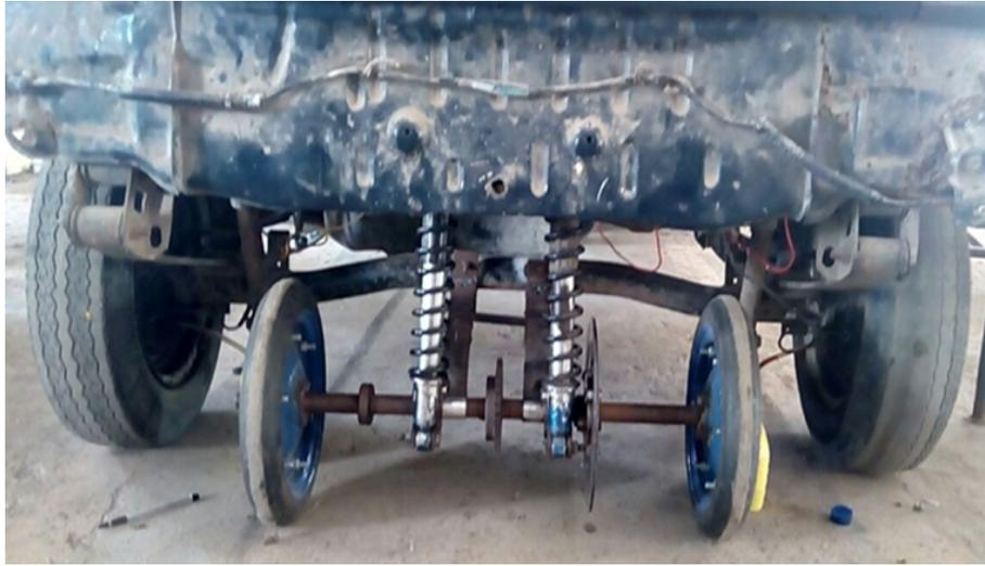
**Figure 1** Sub wheel assembly
