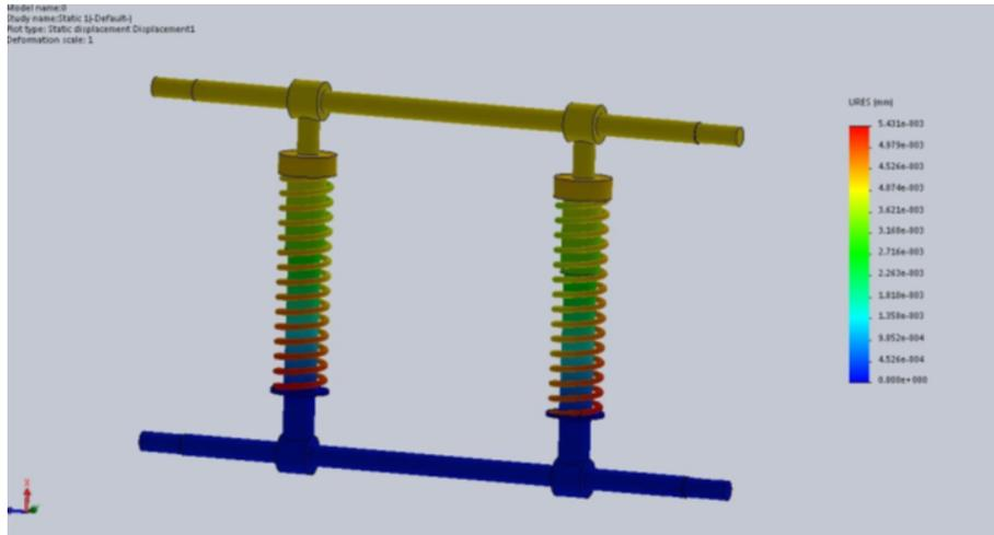
Figure 4 Force analysis with maximum load 400 Kg
