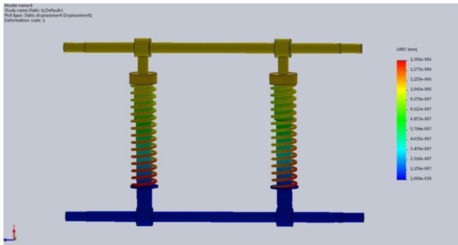
Figure 3 Force analysis with minimum load 200 Kg
