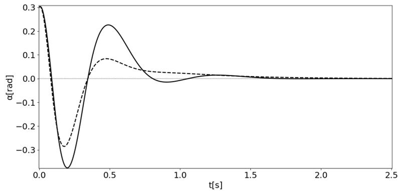
**Figure 4** Stabilization of the pendulum with a controller optimized with respect to  $J$  (solid line) and with a controller that yields the lowest ITAE (dashed line)
