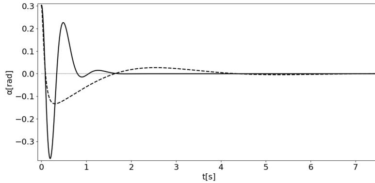
**Figure 3** Stabilization of the pendulum with a controller optimized with respect to  $J$  (solid line) and with a controller that produces the lowest ISE (dashed line)
