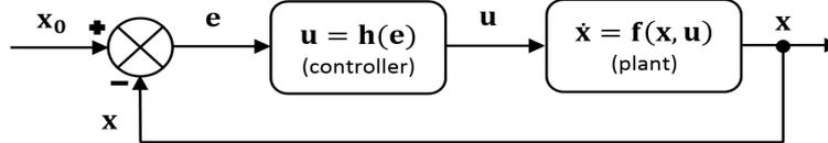
**Figure 1** Scheme of the control system under consideration
