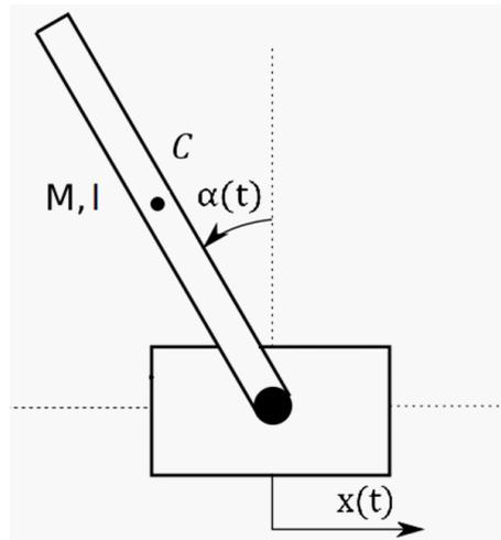
**Figure 2** Sketch of the considered control object – the inverted pendulum
