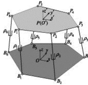
Figure 1 Gough Stewart Platform with notation
