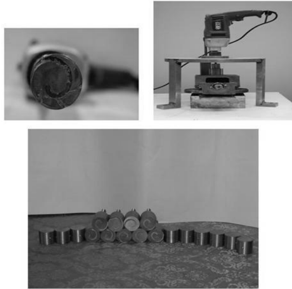
Figure 10 View of the sample (steel washer with the special grooves/notches to catch lubricant actively) – left picture; the test bench – the right picture; the group of samples before testing in the laboratory (below)
