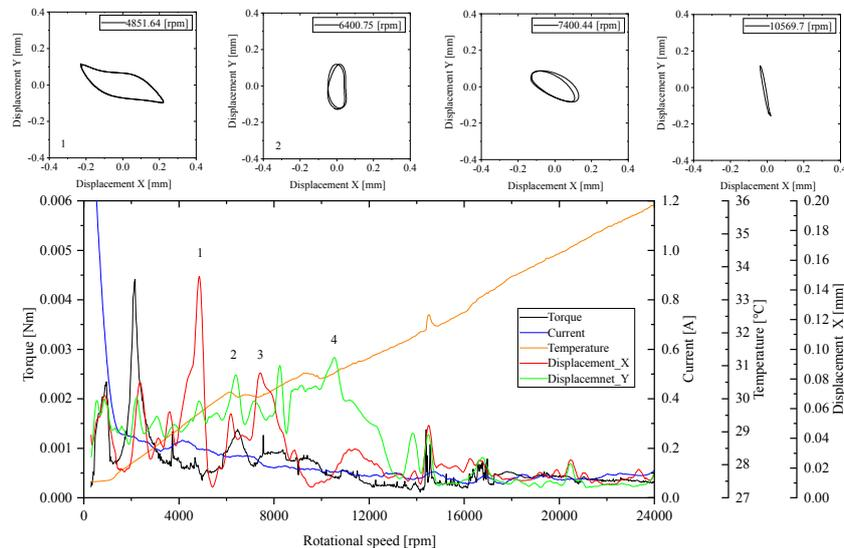
**Figure 5** Torque, electric current, temperature and displacement characteristics as a function of rotational speed recorded during run-up No. 2
