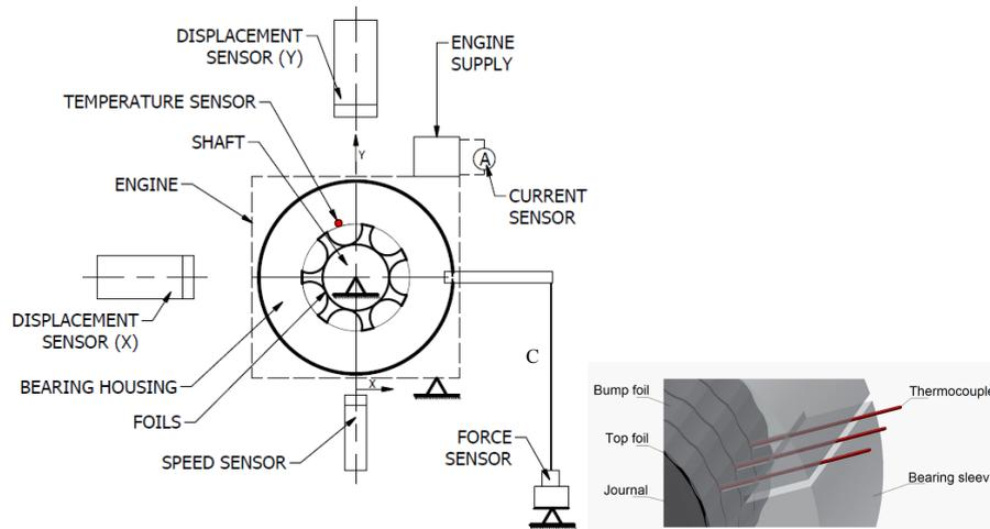
**Figure 1** On the left: Test stand for experimental determination of the lift-off speed of foil bearings. On the right: Arrangement of thermocouples [11]
