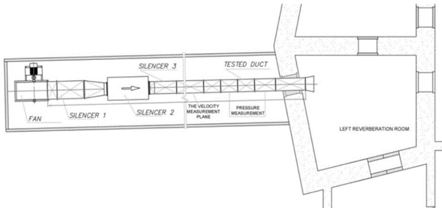
**Figure 2** Construction of test stand with outflow to the reverberation room (according with PN-EN ISO 3741 and PN-EN ISO 7235)
