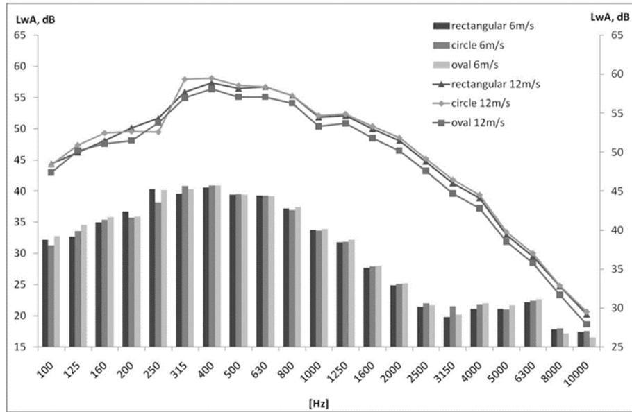
**Figure 3** The 1/3 sound power level with A-correction of studied ducts at 6 m/s (bar graph) and at the 12 m/s (line graph)
