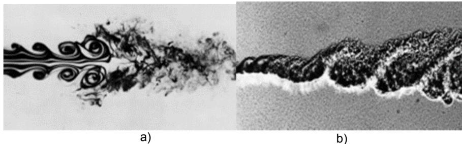
**Figure 1** Flow visualization, effluent in the flooded space: a) the smoke visualization, b) the spark method
