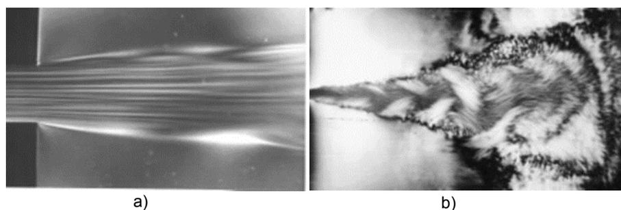
**Figure 2** Visual diagnostics of flow structure: a) the laminar mode, b) the turbulent mode
