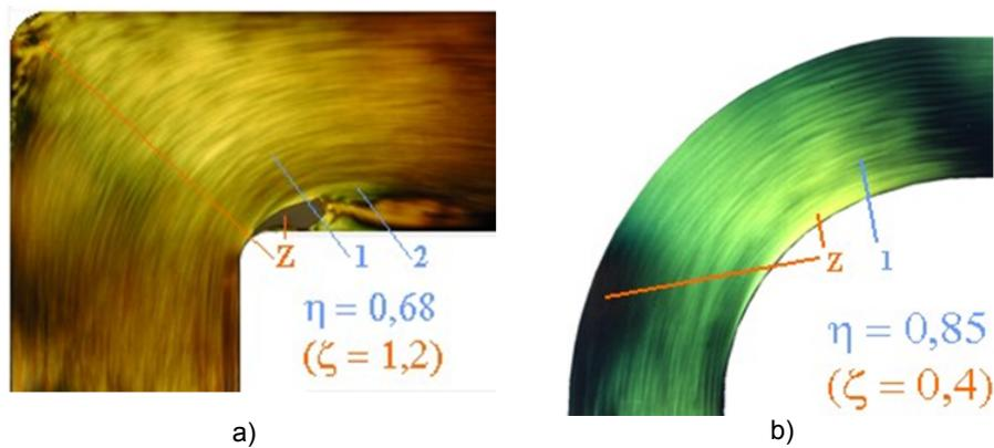
**Figure 3** Flow structure in flow turn by 90°: a) “bend”  $\eta_D = 0,68$ , b) “lateral”  $\eta_D = 0,85$
