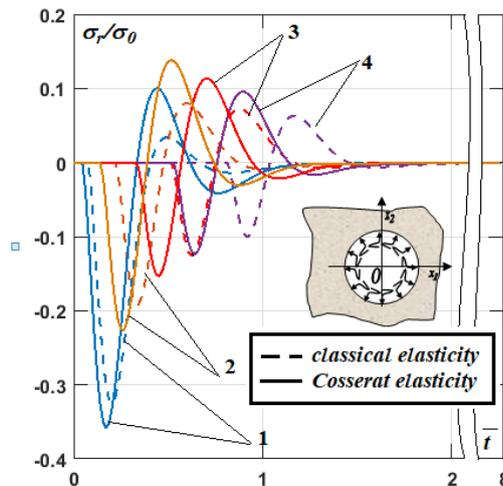
**Figure 3** Relative radial stresses in the polymer foam with tunnel cavity
