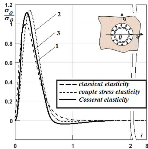
**Figure 2** Relative hoop stresses on the boundary of the cavity in polymer foam
