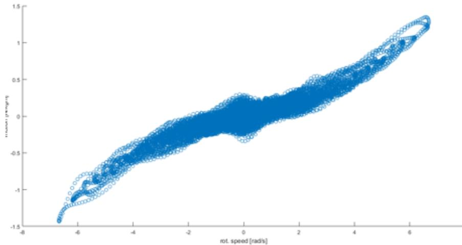
**Figure 5** The experimentally-obtained friction characteristic
