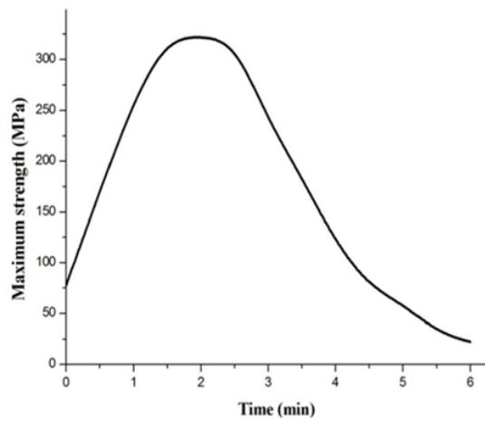
**Figure 4** Tensile strength of unsaturated polyester resin reinforced with etched carbon fibers depending time
