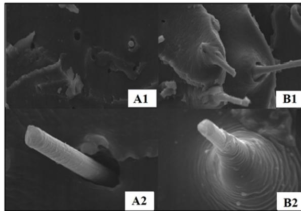
**Figure 2** Fracture surface morphology of unsaturated polyester resin reinforced with A untreated B treated fiber
