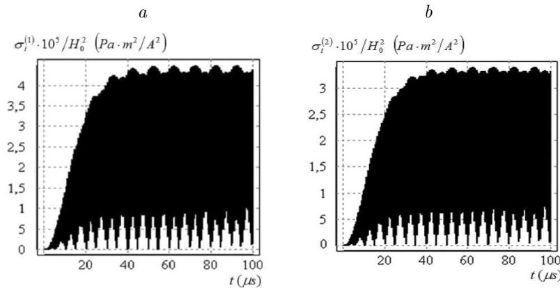
Figure 3 Changes in time of  $\sigma_i^{(n)}$  stresses intensity on the contact surface of steel (a) and copper (b) layer
