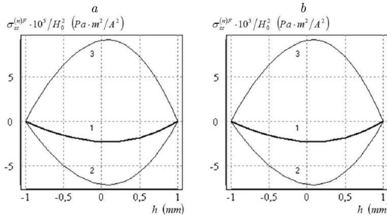
Figure 2 Distribution of  $\sigma_{zz}^{(n)}$  stresses (a, b) in the thickness of bimetallic plate at different moments
