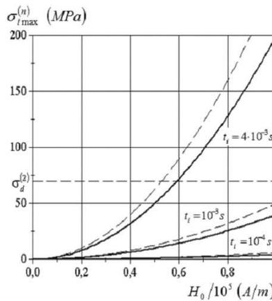
**Figure 5** Dependence of the maximal values of  $\sigma_{i \max}^{(n)}$  on values of  $H_0$  for different pulse durations
