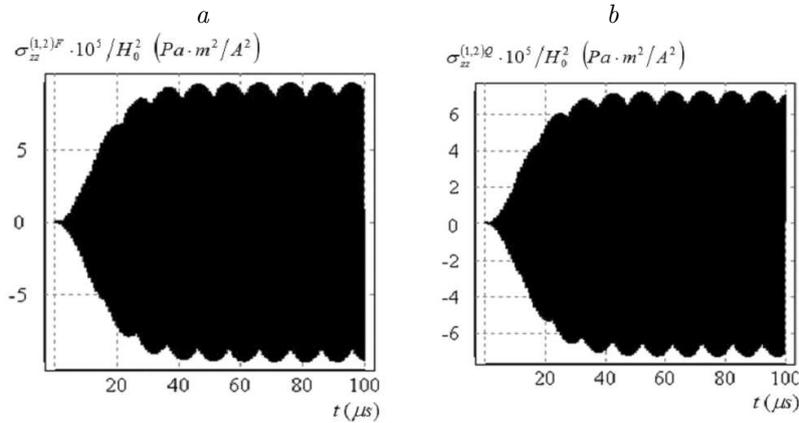
Figure 1 Variation in time of  $\sigma_{zz}^{(n)}$  stresses (a, b) on the contact surface
